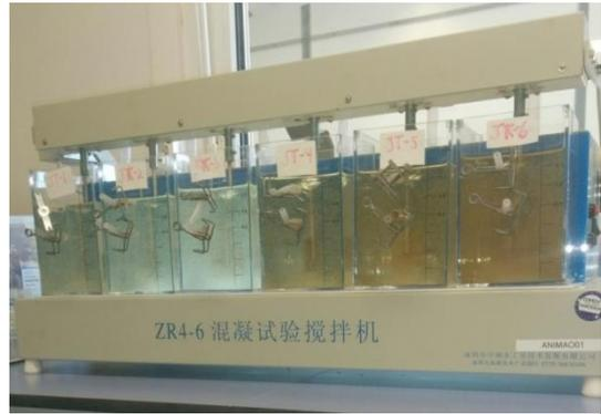
Figure 13: Shenzhen ZR4-6 jar tester
