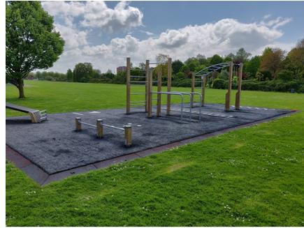
(a) The plug and play playgrounds have interchangeable pieces of play equipment that have a standardized footprint. Equipment can be changed while keeping the same foundations. These parks have large open spaces in between the large, wooden pieces of equipment.
