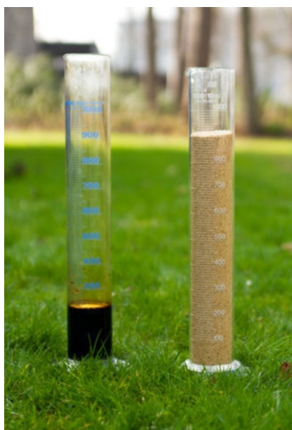
Figure 2.1: Pyrolysis oil (left) and pinewood from which it originates (right). Both cylinders contain the same amount of energy, showing that during pyrolysis the volumetric energy content increased considerably [42].
