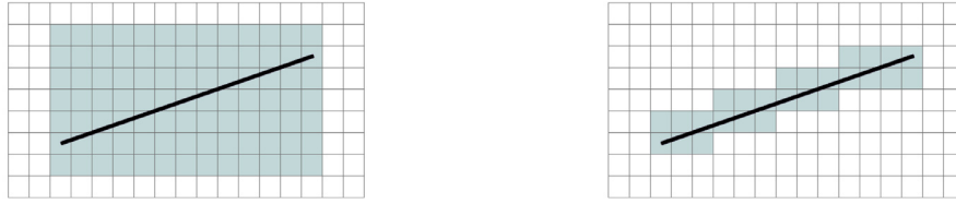
(a) Cell selection A: rectangular domain enclosing the VG. (b) Cell selection B: cells aligned with the VG.
