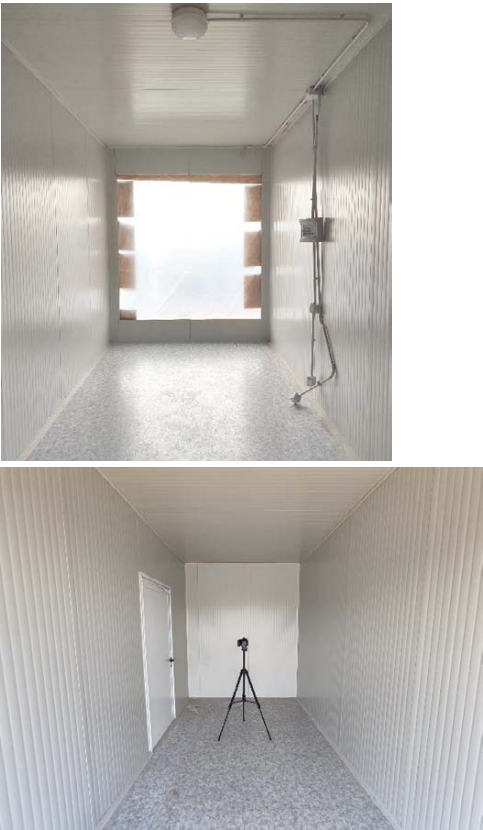
Figure 7: Placement of the luminance photometer within one of the test cells (no glazing installed)
