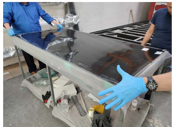
Figure 6: Placement of films in between the interlayers prior to lamination.
