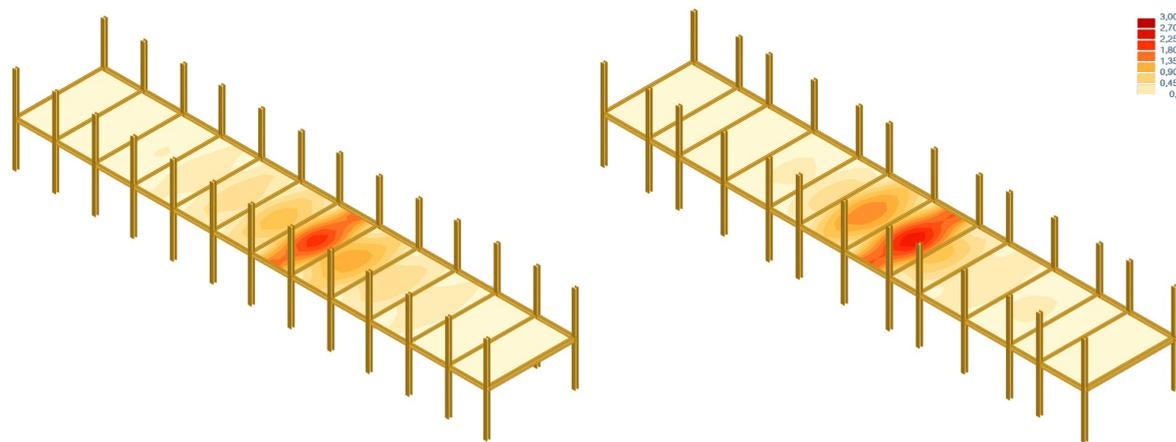
(a) Triple 2.7 meter bay span,  $v_{RMS}$  (2,18-1,29)
