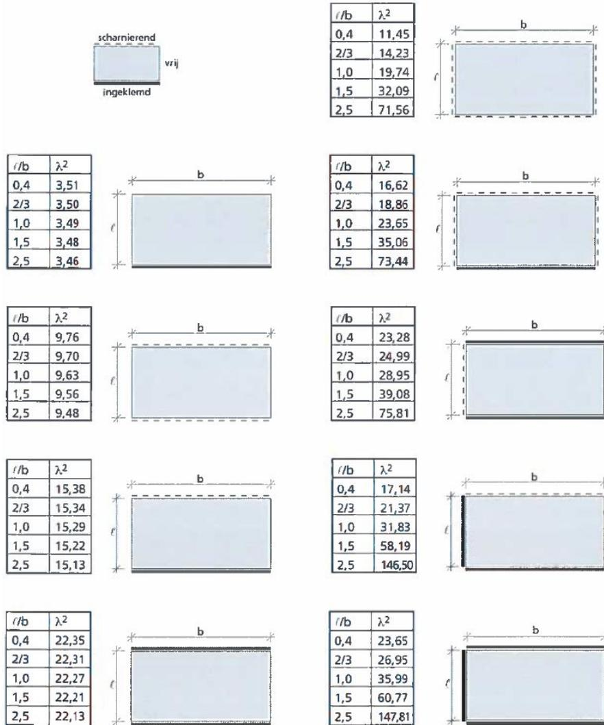
Figure A.1: Eigenfrequencies of floor plates [36].
