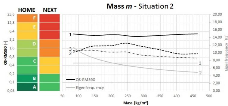
Figure 4.42: OS-RMS<sub>90</sub> and natural frequency for alternating mass (situation 2).
