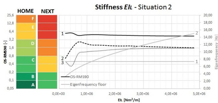
Figure 4.34: OS-RMS<sub>90</sub> and natural frequency for alternating floor stiffness (situation 2).
