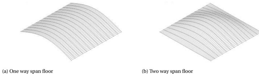
Figure 4.2: First mode shapes for two different floor systems.
