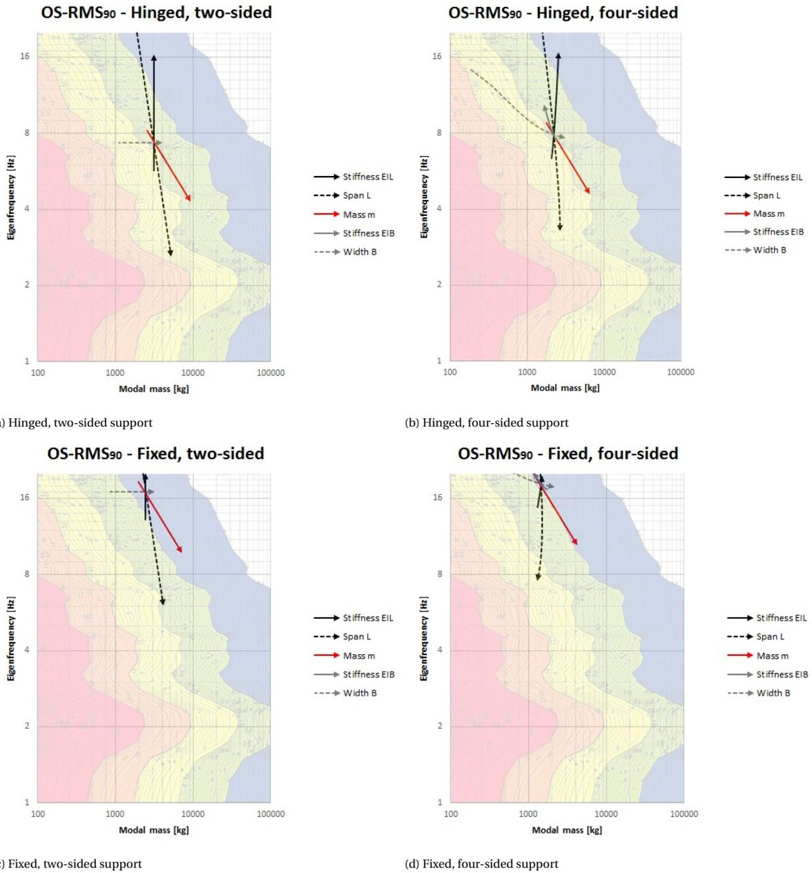
Figure 4.16: OS-RMS<sub>90</sub> chart with varying properties for different support conditions.
