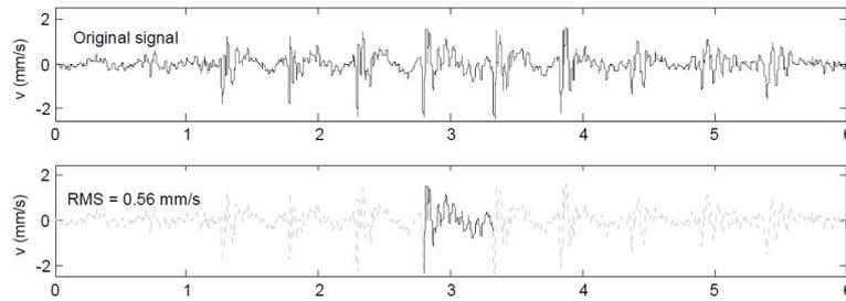
Figure 3.2: Velocity-time response of a floor imposed to walking loads for complete path (up) and one step (down) [9].
