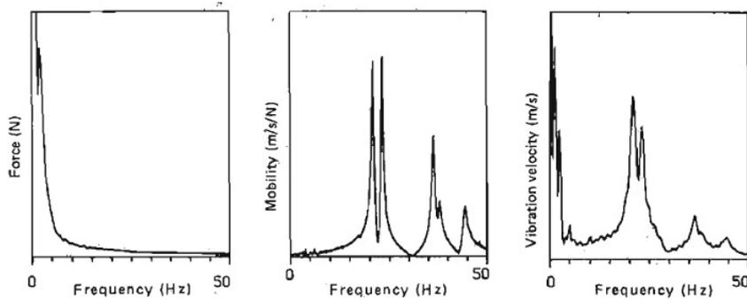
Figure 3.10: Footstep force, mobility of the structure and resulting vibrating velocity [29].
