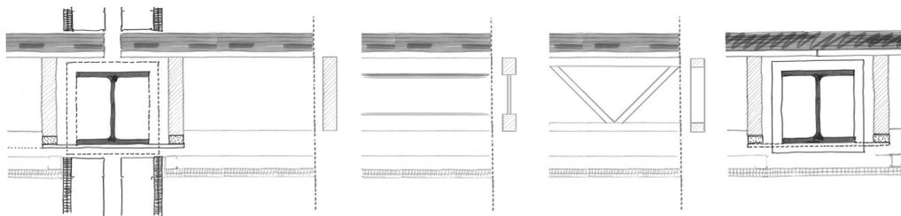
Figure 5.4: Schematic depiction of various joist profiles (resp. solid, I-joist and open-web).
