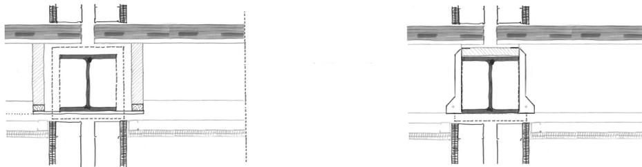
Figure 5.15: Schematic depiction of joist to beam fixation (resp. without and with bearings).
