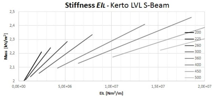
Figure B.1: Stiffness to mass ratio for various rectangular joist profiles.
