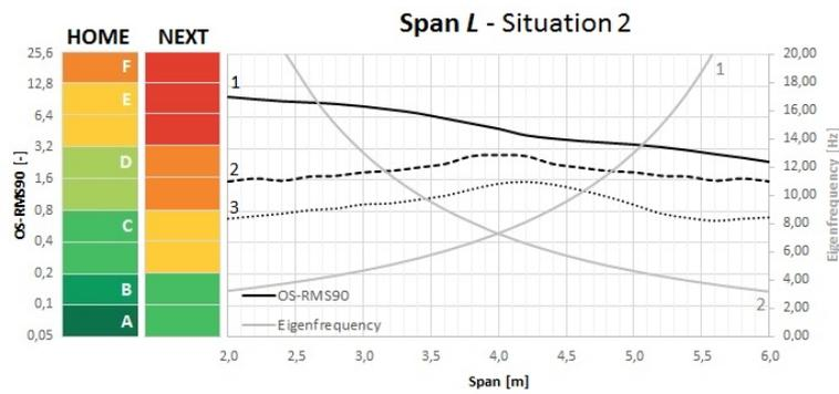
Figure 4.38: OS-RMS<sub>90</sub> and natural frequency for alternating floor spans (situation 2).
