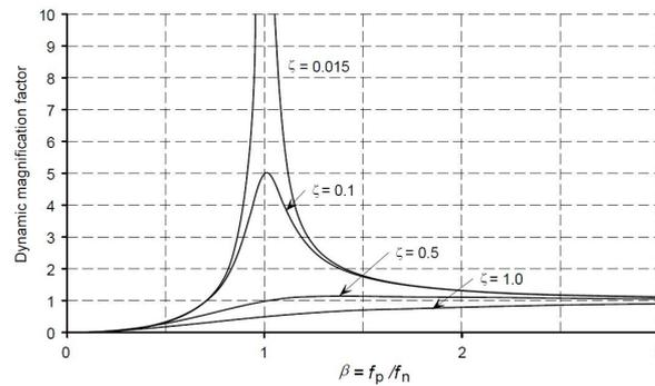
Figure 3.7: Dynamic magnification factor for different damping levels [32].
