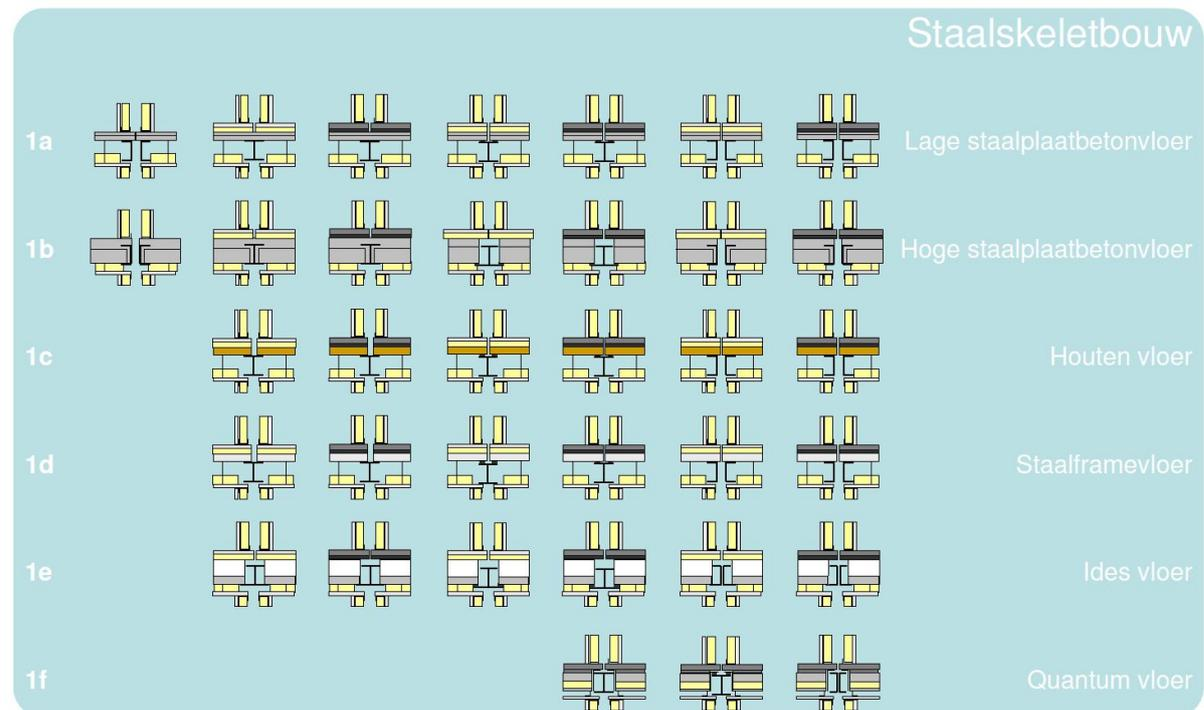
Figure 2.4: Steel framing with light-weight floors schematic junctions [33].
