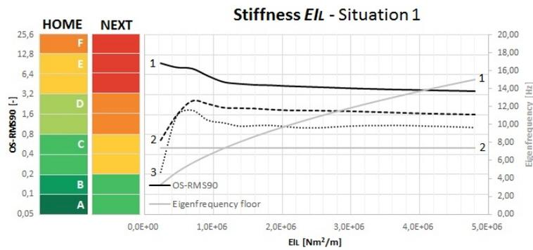
Figure 4.33: OS-RMS<sub>90</sub> and natural frequency for alternating floor stiffness (situation 1).
