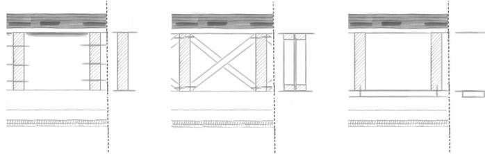
Figure 5.6: Schematic depiction of various transverse bridging (resp. solid blocking, cross-bridging and strapping).
