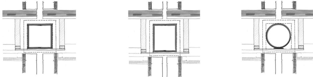
Figure 5.13: Schematic depiction of various hollow section profiles (resp. SHS, RHS and CHS).
