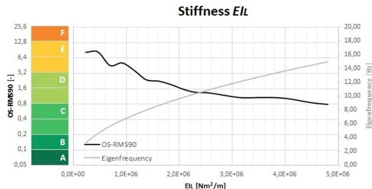
Figure 4.10: OS-RMS<sub>90</sub> and natural frequency for varying stiffness.
