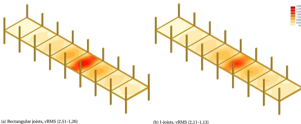
Figure 5.5: Footfall analysis for different type of floor joists.
