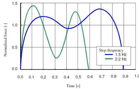
Figure 3.3: Load-time function of a single step for certain step frequencies [9].
