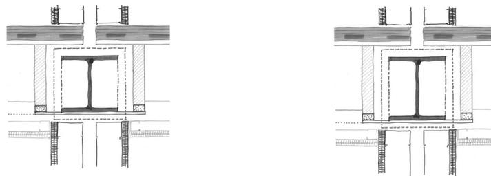
Figure 5.11: Schematic depiction of various H-beam profiles (resp. HEA220 and HEA300).
