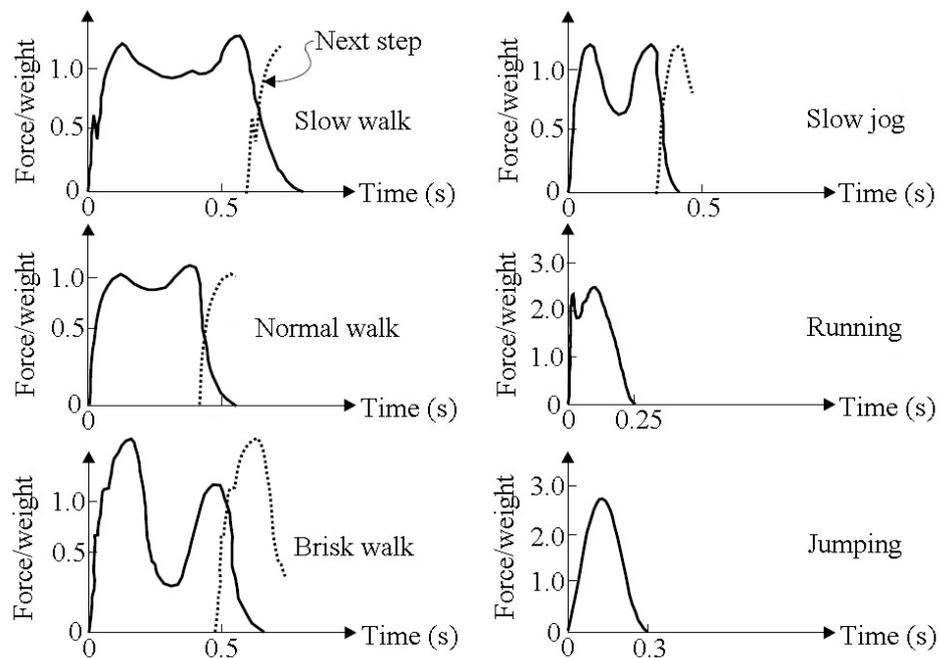
Figure 3.4: Load-time functions for different activities [38].
