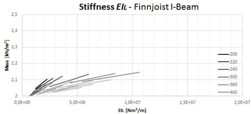
Figure B.2: Stiffness to mass ratio for various I-joist profiles.
