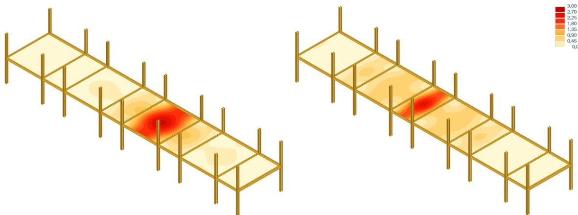
(a) Alternating 5.0-3.0 meter bay span,  $v_{RMS}$  (2,80-0,74)
