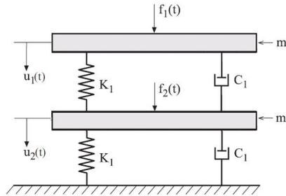
Figure 3.6: Mass-spring-damper MDOF system.
