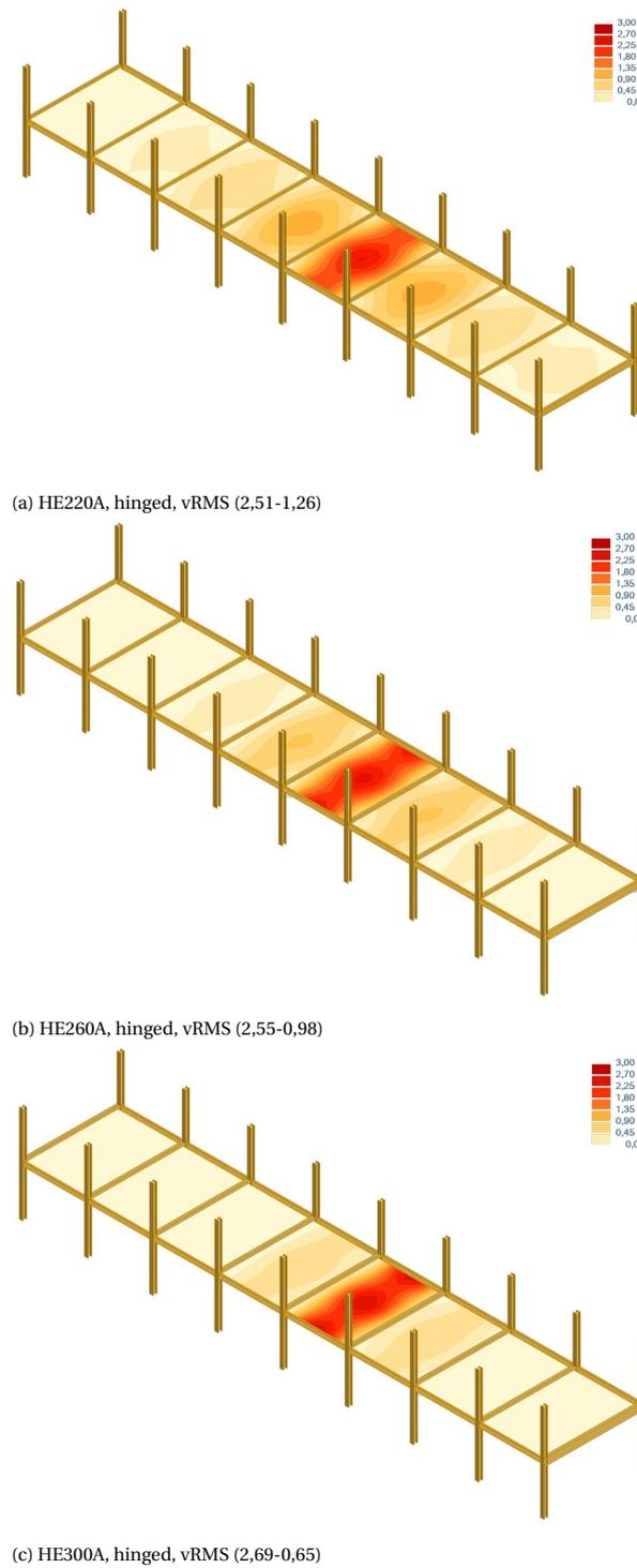
Figure 5.12: Footfall analysis, various HEA beam profiles.
