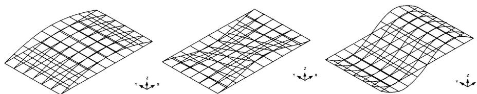
Figure 3.8: First three mode shapes for a two sided supported floor [24].
