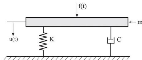
Figure 3.5: Mass-spring-damper SDOF system.
