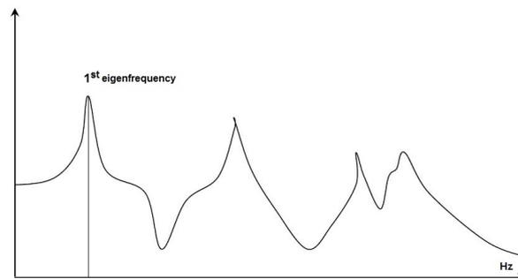
Figure 4.18: MDOF admittances spectrum in the frequency domain [19].
