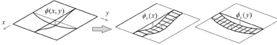
Figure 3.9: Approximated mode shape of orthotropic floor supported on four sides [18].
