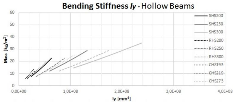
Figure B.5: Bending stiffness to mass ratio for various hollow beam profiles.
