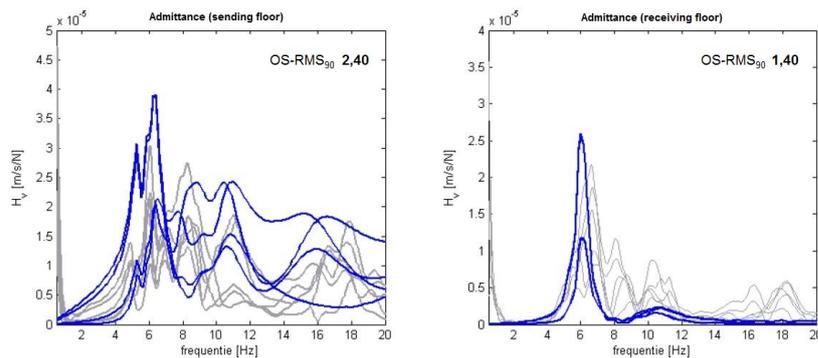
Figure 4.19: Admittances from measurements 'De Karel Doorman' [19].
