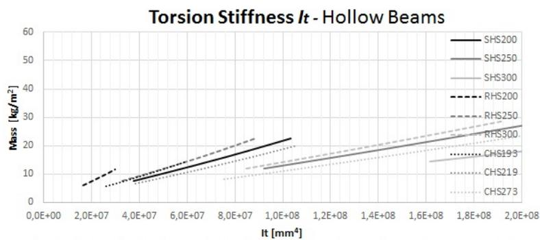
Figure B.6: Rotational stiffness to mass ratio for various hollow beam profiles.
