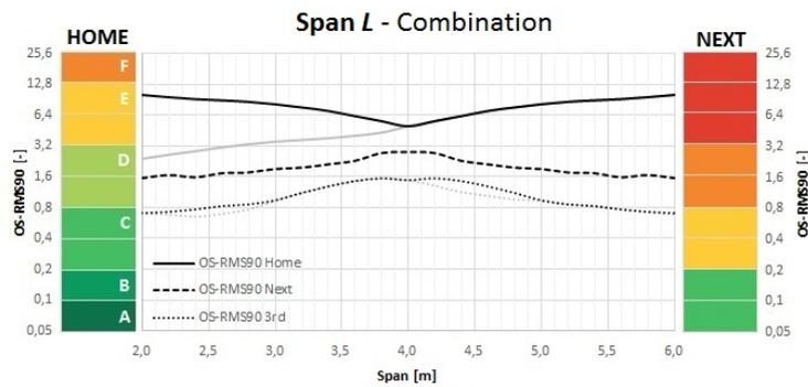
Figure 4.39: OS-RMS<sub>90</sub> for alternating floor spans (combined).
