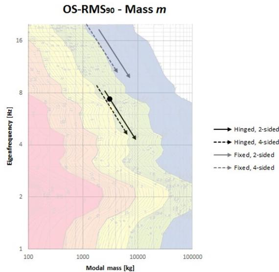
Figure 4.13: OS-RMS<sub>90</sub> chart with varying mass for different support conditions.
