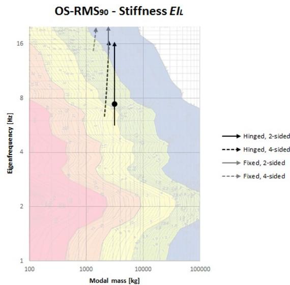
Figure 4.9: OS-RMS<sub>90</sub> chart with varying stiffness for different support conditions.
