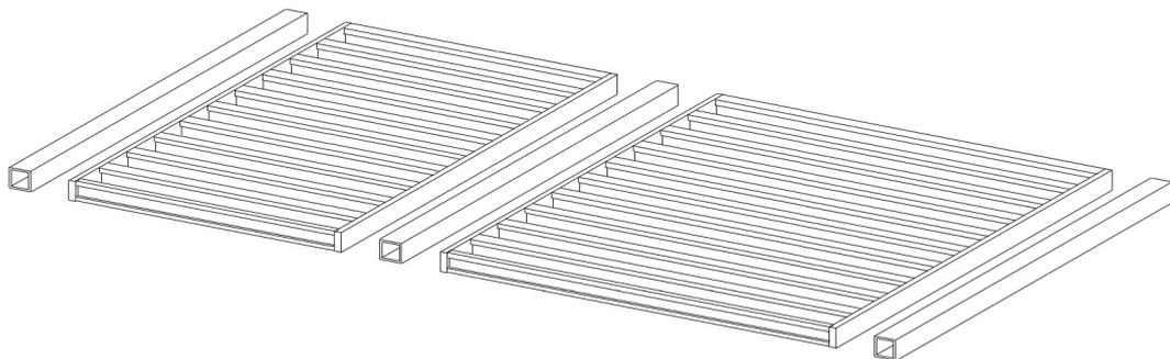
Figure 6.6: Schematic build-up alternating span concept.
