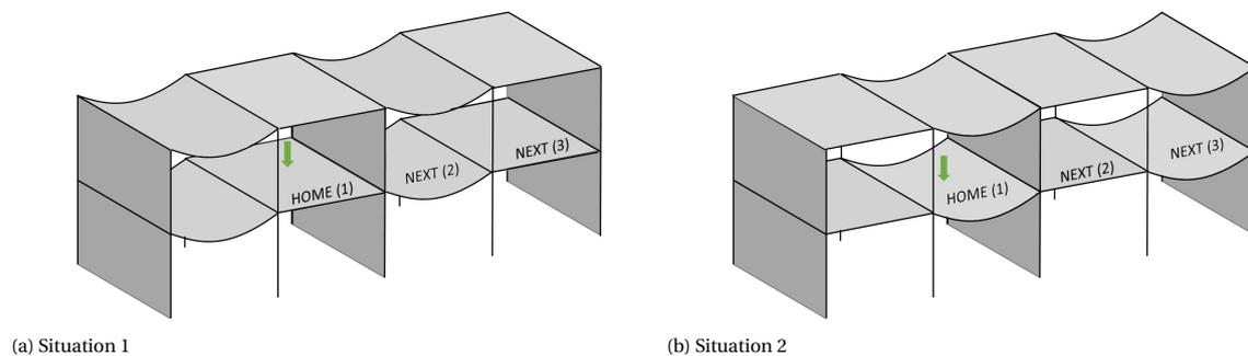
Figure 4.32: Alternating stiffness situations.
