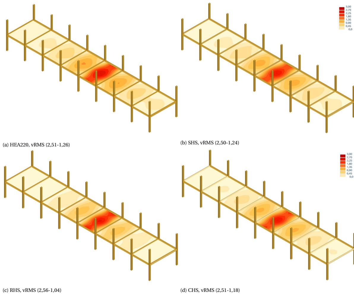
Figure 5.14: Footfall analysis, various hollow section beam profiles.
