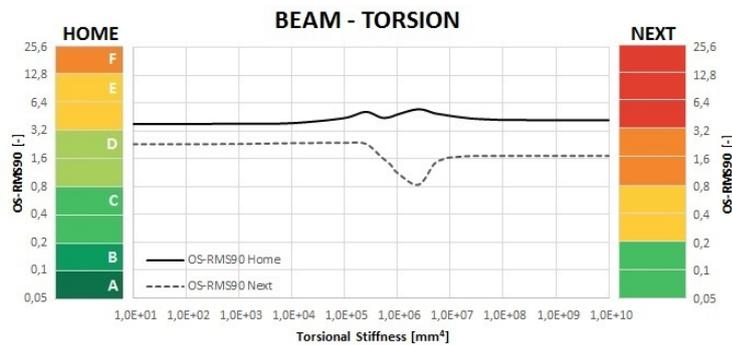
Figure 4.31: OS-RMS<sub>90</sub> for varying torsion stiffness beam.
