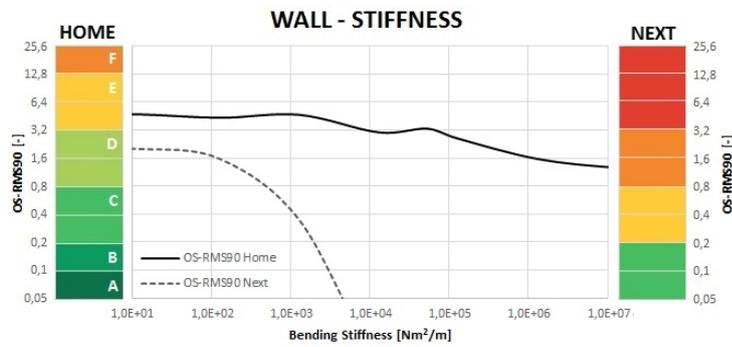
Figure 4.29: OS-RMS<sub>90</sub> for varying wall stiffness.
