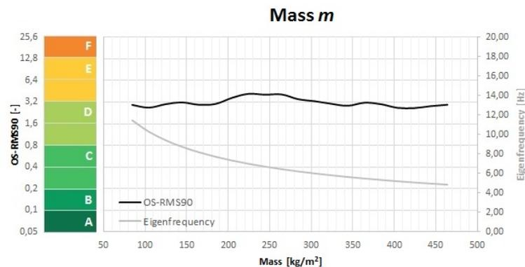
Figure 4.14: OS-RMS<sub>90</sub> and natural frequency for varying mass.
