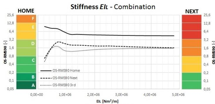
Figure 4.35: OS-RMS<sub>90</sub> for alternating floor stiffness (combined).
