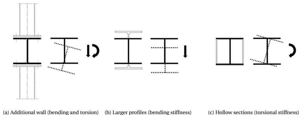
Figure 4.28: Schematic representation of junction adjustments.
