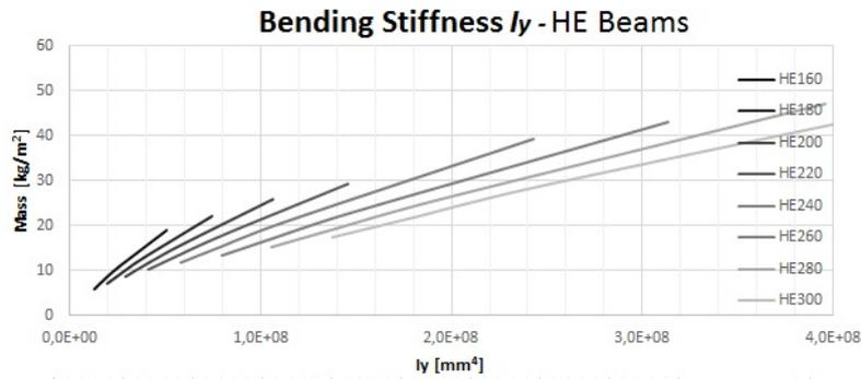
Figure B.3: Bending stiffness to mass ratio for various HE beam profiles.
