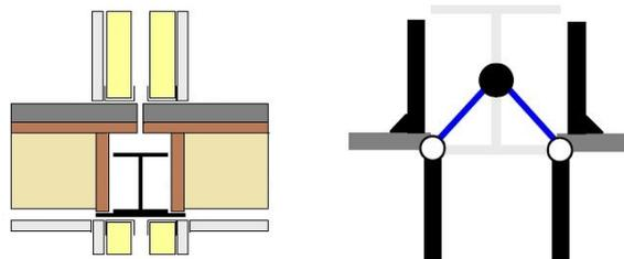
Figure 4.7: Schematic junction of 'De Karel Doorman' [33].
