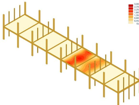
Figure 5.18: Footfall analysis, added stiffness in walls.
