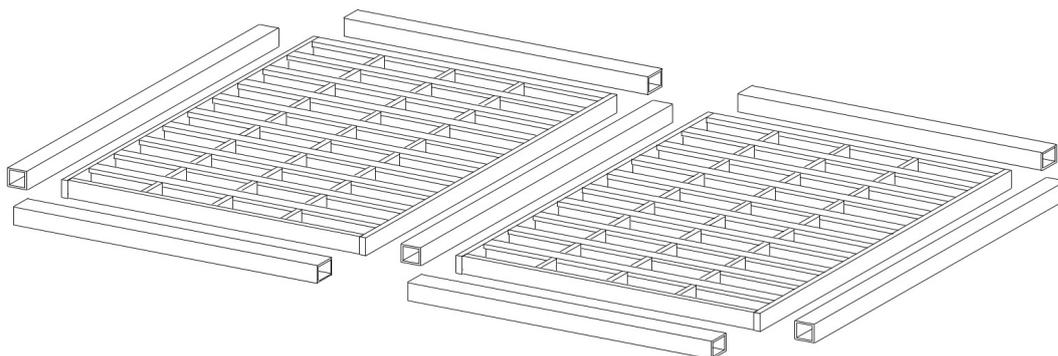
Figure 6.5: Schematic build-up two-way span concept.
