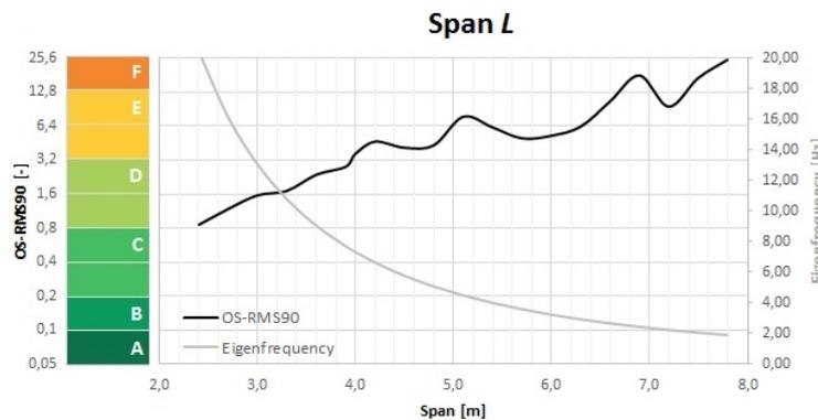
Figure 4.12: OS-RMS<sub>90</sub> and natural frequency for varying span.
