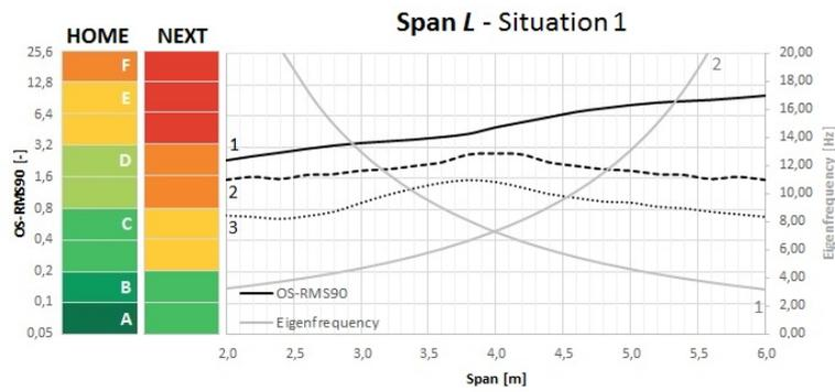
Figure 4.37: OS-RMS<sub>90</sub> and natural frequency for alternating floor spans (situation 1).
