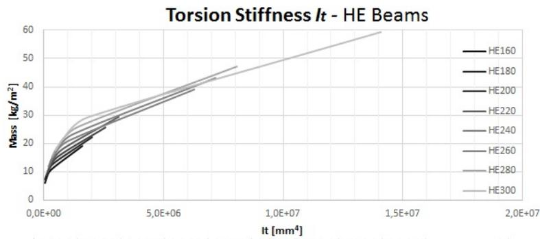
Figure B.4: Rotation stiffness to mass ratio for various HE beam profiles.
