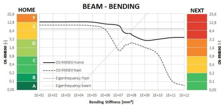
Figure 4.30: OS-RMS<sub>90</sub> for varying bending stiffness beam.
