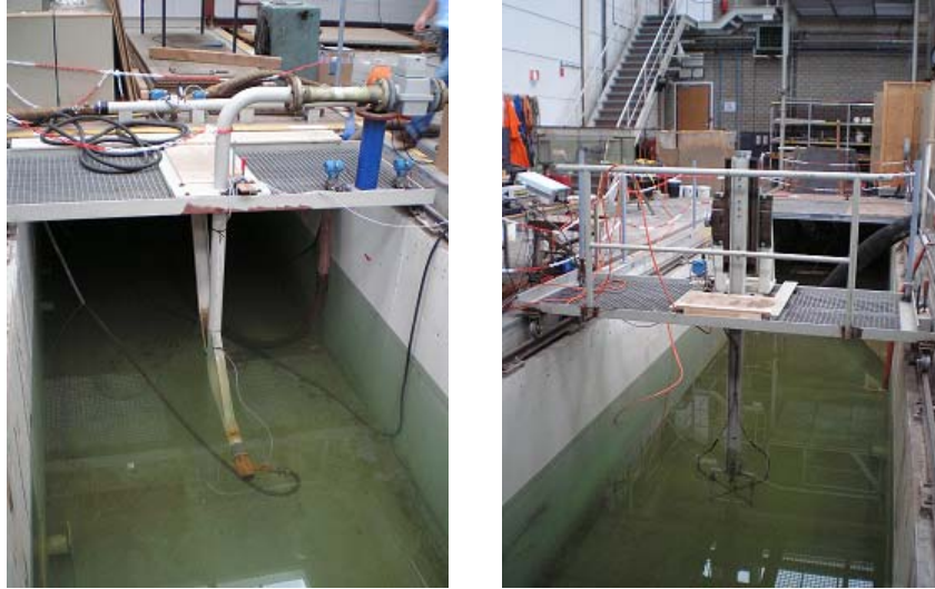
Figure 31 the fixed construction of the water jet (left) and the carriage with measuring probes (right).
