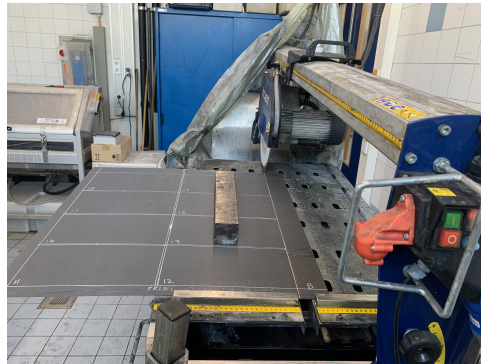
Figure G.7: Laminate cutting with diamond saw
