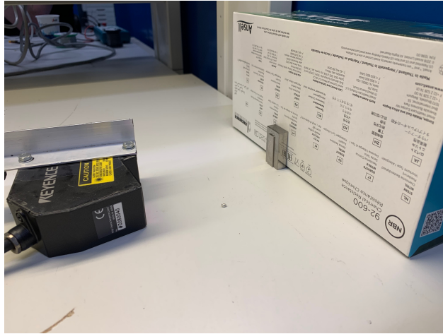
Figure D.5: Calibration of the LDS
