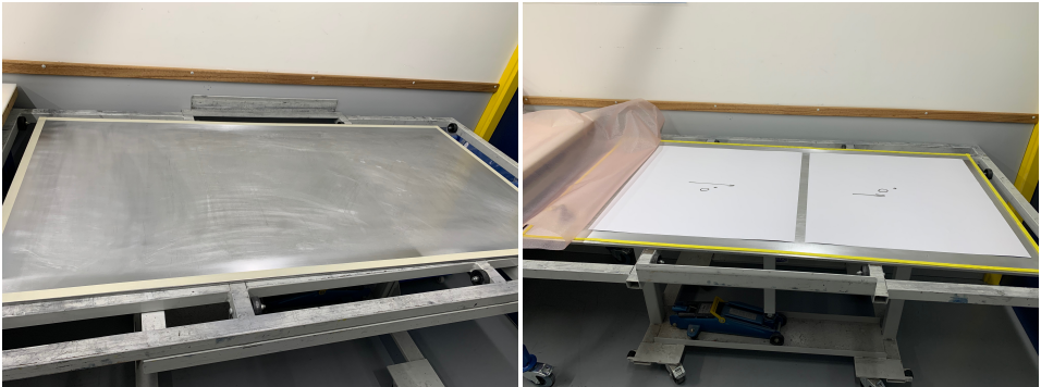
Figure G.3: Autoclave plate and hand layup process
