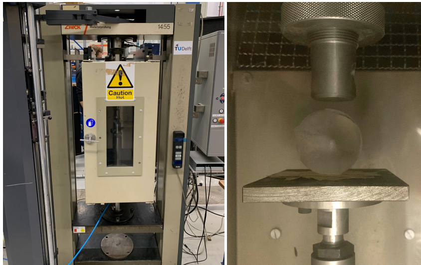
Figure 4.2: Zwick 20kN UTM with the temperature control chamber
