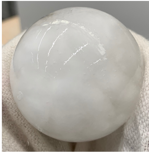
Figure 4.5: SHI with cotton at 10% weight fraction
