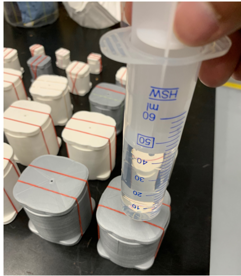
Figure 4.1: Filling of moulds with distilled water using a syringe
