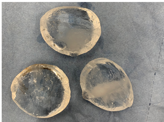
Figure B.1: Pure SHI after compression test
