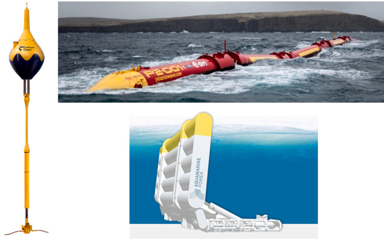
Fig. 1. The WECs used within this study are (a) PA inspired by C4 Corpower (left), (b) Pelamis (right top), and (c) Flat-type (right bottom).
