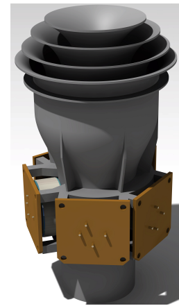
Figure 4.2: Rendering of the channel with all sensors and sensor boards attached
