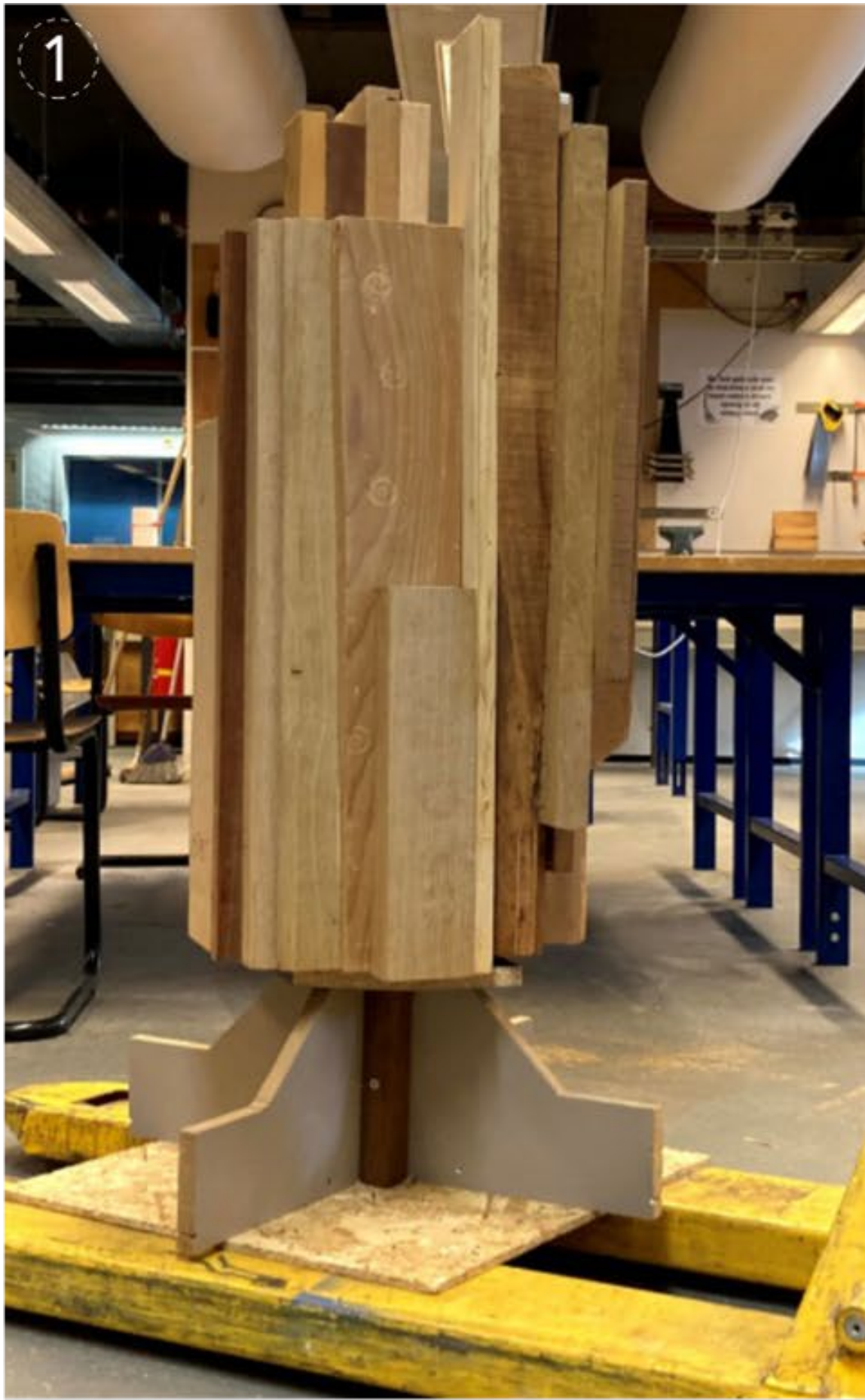
Recycled Wood is packed and glued together to form one monolithic block
