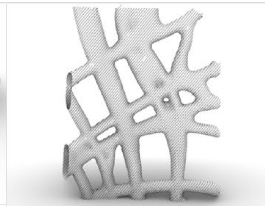
Changing the Orientation of the segment 3D printing at 45° angle
