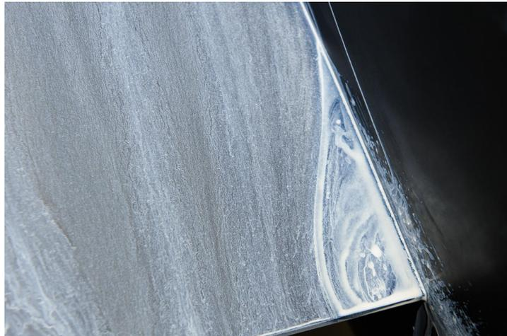
Figure 2.6: Oil-flow visualisation of the corner separation at a pitch angle of 5 degrees of the NASA experiment. Kegerise et al.;
