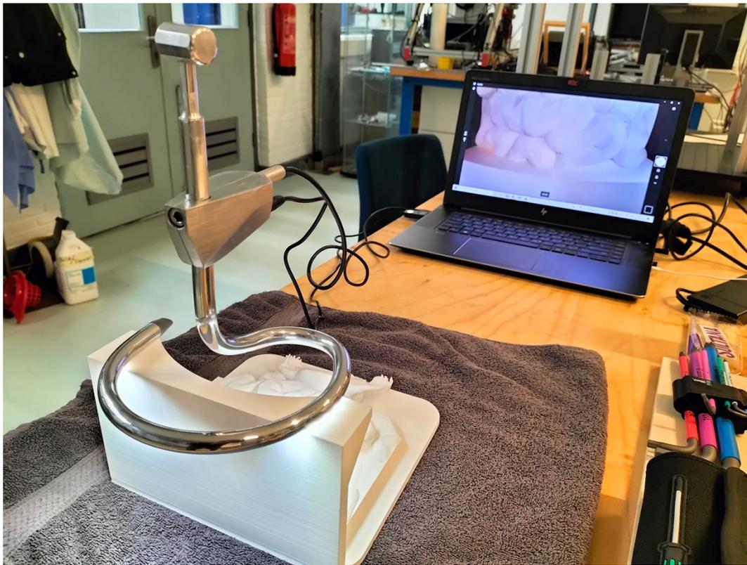
**Figure 11.9:** The aluminium prototype imaging a 3D-printed intestinal model.
