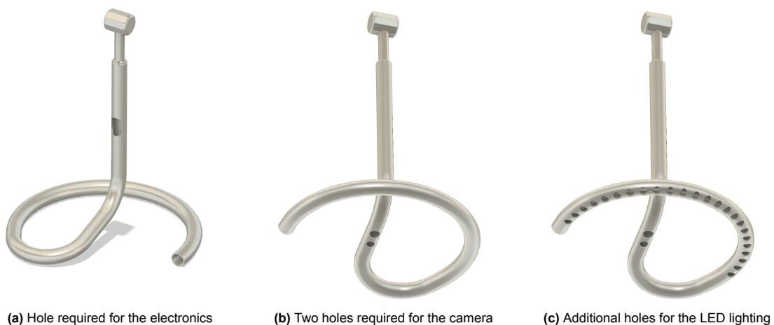
**Figure 9.3:** The three sites where holes in the structure are required.
