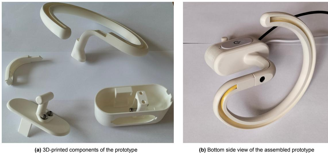
**Figure 11.2:** Overview of the fourth-generation 3D-printed prototype.
