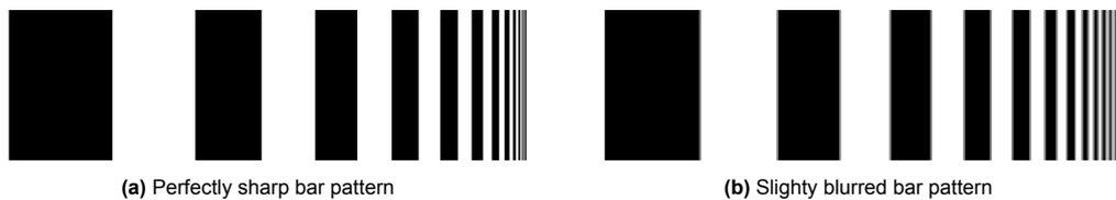
Figure 12.2: Example bar pattern, original and with camera degradation.
