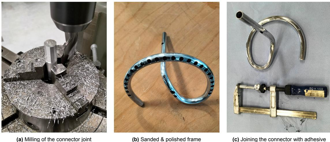
(a) Milling of the connector joint
