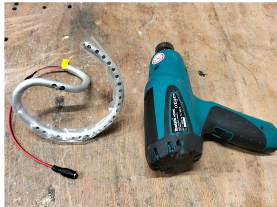
(b) Test frame used to determine total illuminance
