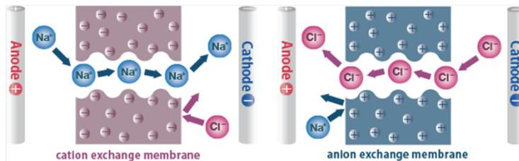
Figure 2: Ion exchange membranes. Due to the negatively charged fixed ion groups of a CEM, cations permeate easily while anions are impeded. The reverse is true for an AEM. [6]
