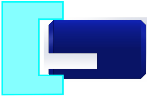
Figure 6.7: Pre-stress idea by using a dowel pin with a slot cut in. The top side provides a reference surface, while the bottom side provides a spring force to the flexure. The flexure hole is not quite circular, but has a slightly decreased radius at the bottom so it interferes with the dowel pin.
