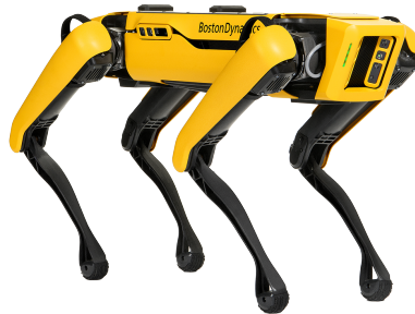
Figure 2-3: The used agent for this research, Spot by Boston Dynamics.
