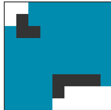
(b) After a full scan of the environment, the blue area is returned by Bresenham's algorithm
