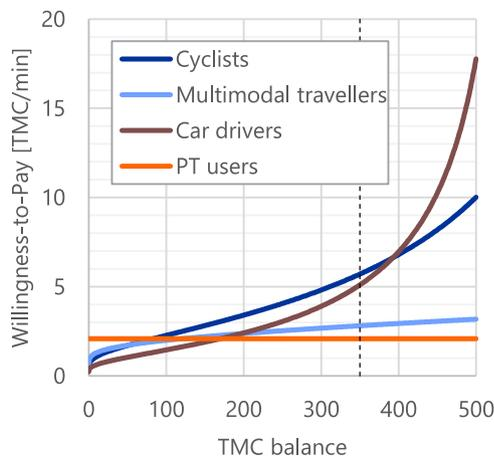
Fig. 11. Willingness-to-Pay for travel time improvements, given the TMC balance.
