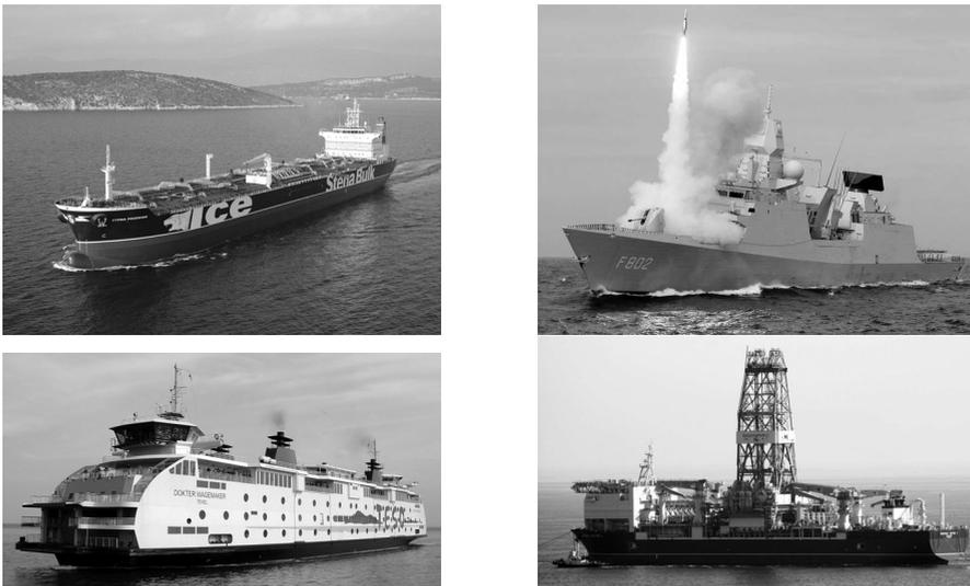
**Fig. 1.1** – Two transport vessels: an oil tanker (upper-left) and car ferry (lower-left) and two service vessels: a frigate (upper-right) and a deep water drillship (lower-right)
