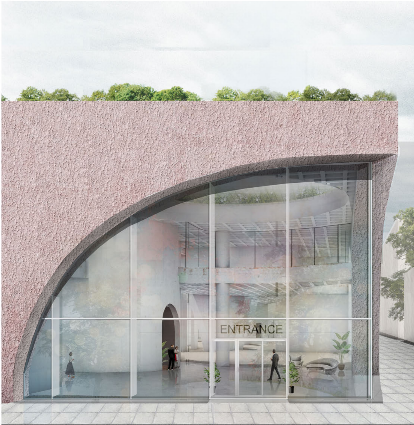
The concrete facade also functions as an important load bearing structure.
