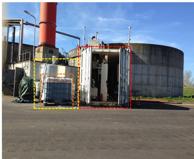
Fig. 1. Impression of the pilot plant. The open container contained the selector and accumulator bioreactor (red bracket). In the front, there is an IBC sedimentation tank (orange bracket). Behind the sedimentation tank, the influent buffer vessel was located (yellow bracket). (Image by Michel Mulders.)
