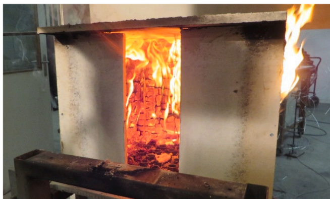
Fig. 12. Compartment 2.2 with three CLT walls remained in flaming combustion due to fall-off of charred lamellae after the initial fire was stopped.
