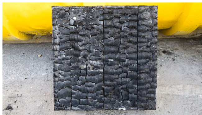
Fig. 14. No fall-off of charred lamellae had occurred.
