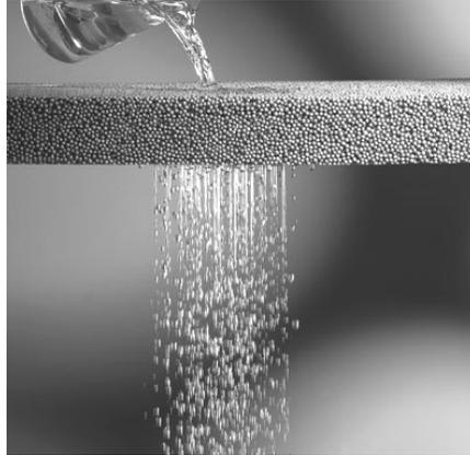
*Figure 5.26 Water can flow through the pore spaces of a material (BrockUSA, 2008).*
