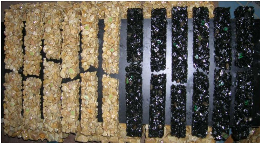
Figure 5.20 Breaking positions of beams tested in three-point bending test (Gu, 2007b).
