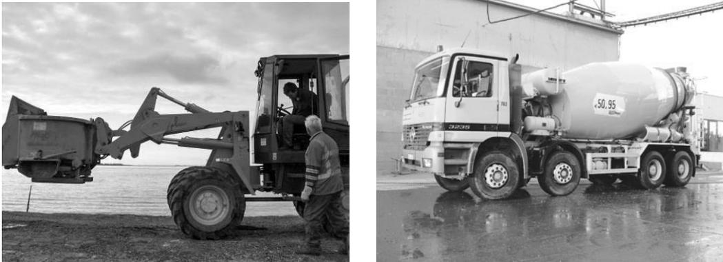
*Figure 3.3 Specially equipped shovel capable of tumbling and dumping (left) and standard concrete mixing truck (right).*
