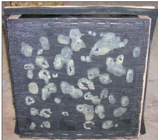
*Figure 3.5 Leaking of superfluous polyurethane adhesive on the underlying geotextile of an Elastocoast cube sample (Gu, 2007).*
