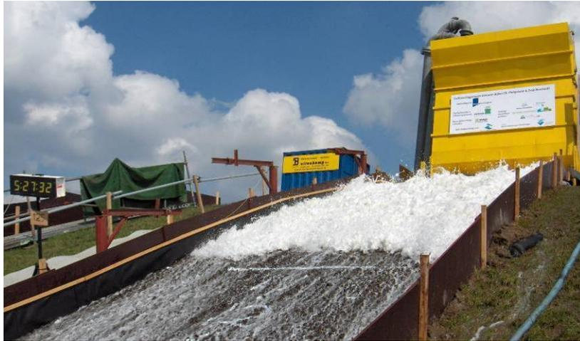
Figure 1.6 Overtopping test at Kattendijke (NL). Waves were simulated to create overtopping volumes of up to 125 l/s/m.
