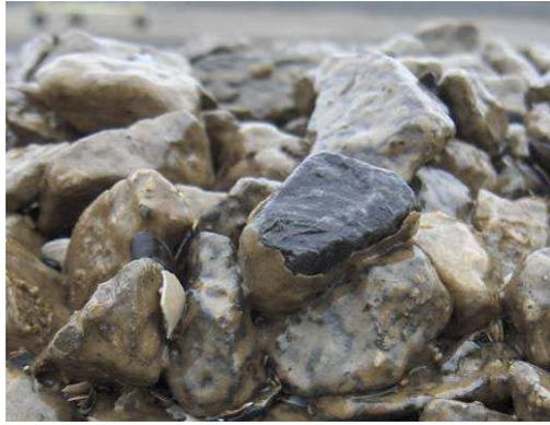
Figure 6.3 Signs of the use of moist aggregate during construction: light discoloration and stripping of the polyurethane film.
