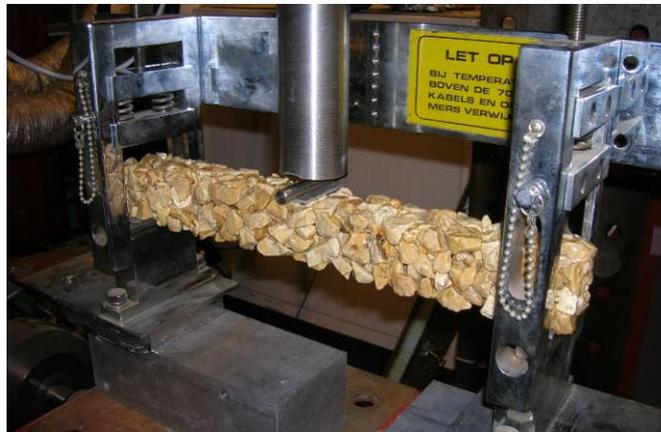
Figure 1.7 Three point bending test on an Elastocoast beam (Gu, 2007).
