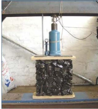
Figure 3.14 Compression test with an Elastocoast cube sample (Pasche, 2007).
