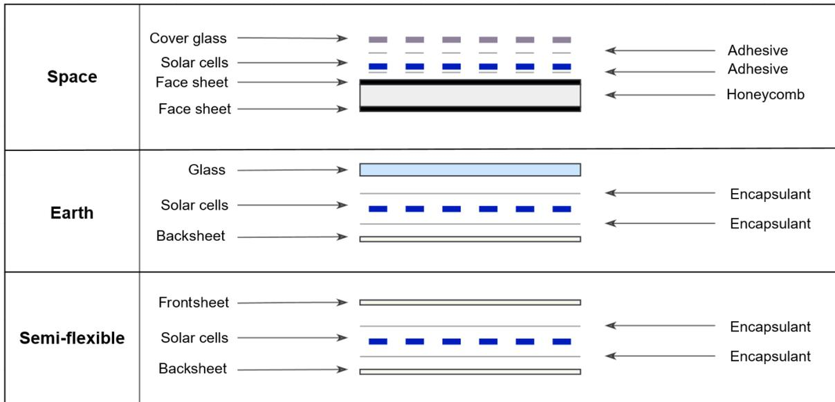
Figure 3.1: Schematic visualization of different types of solar panels
