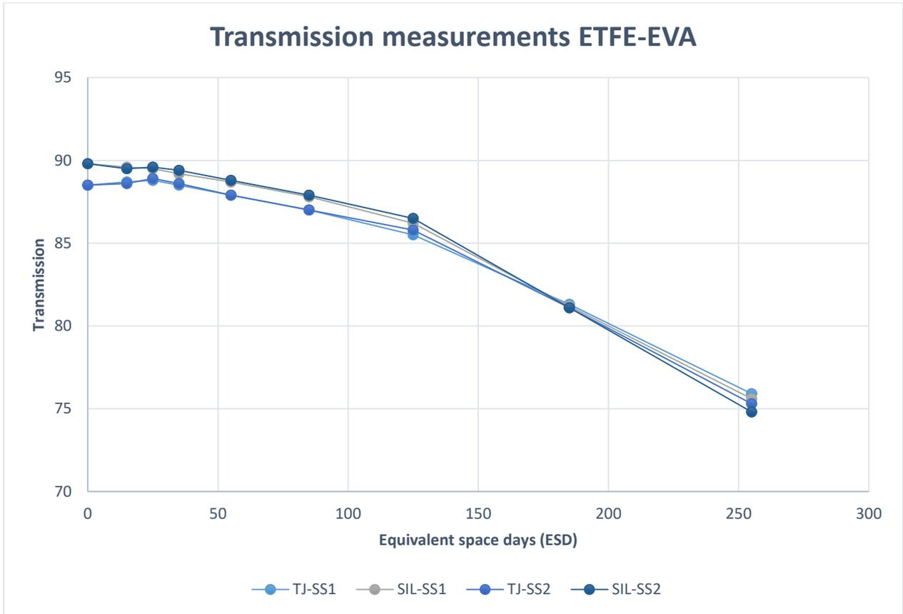
Figure 7.5: Transmission of ETFE sample for a TJ and a Silicon cell as a result of VUV degradation
