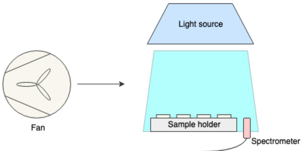
Figure 6.7: Schematic representation of VUV degradation experimental setup
