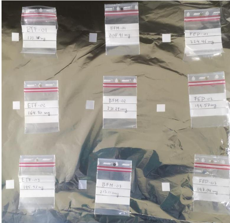
Figure 6.12: Outgassing samples before entering the vacuum oven
