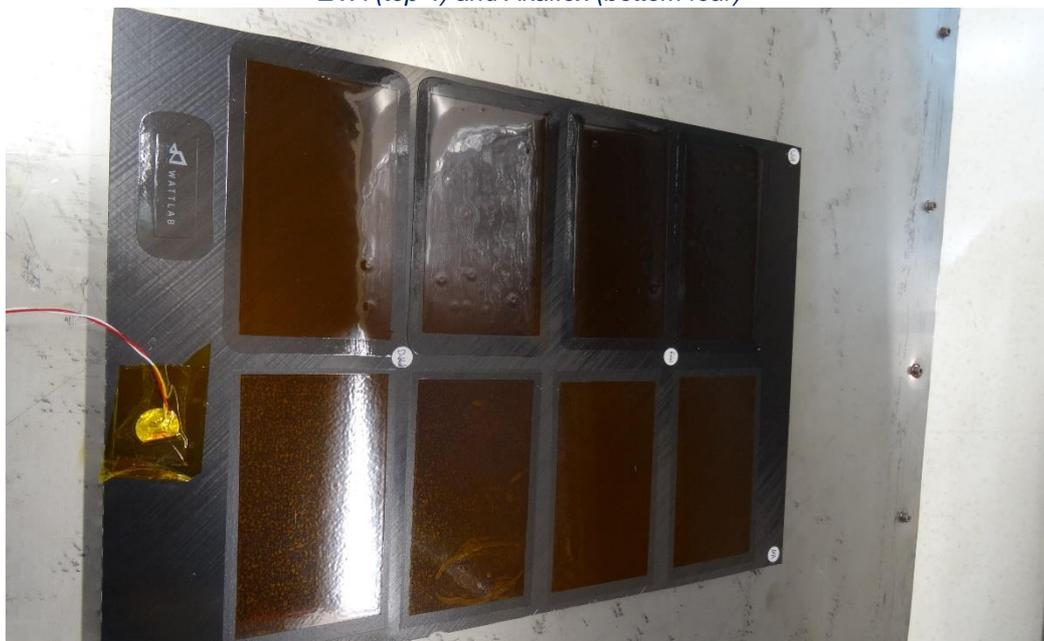
Figure A.13: Bonding of kapton on carbon face sheet smooth side
