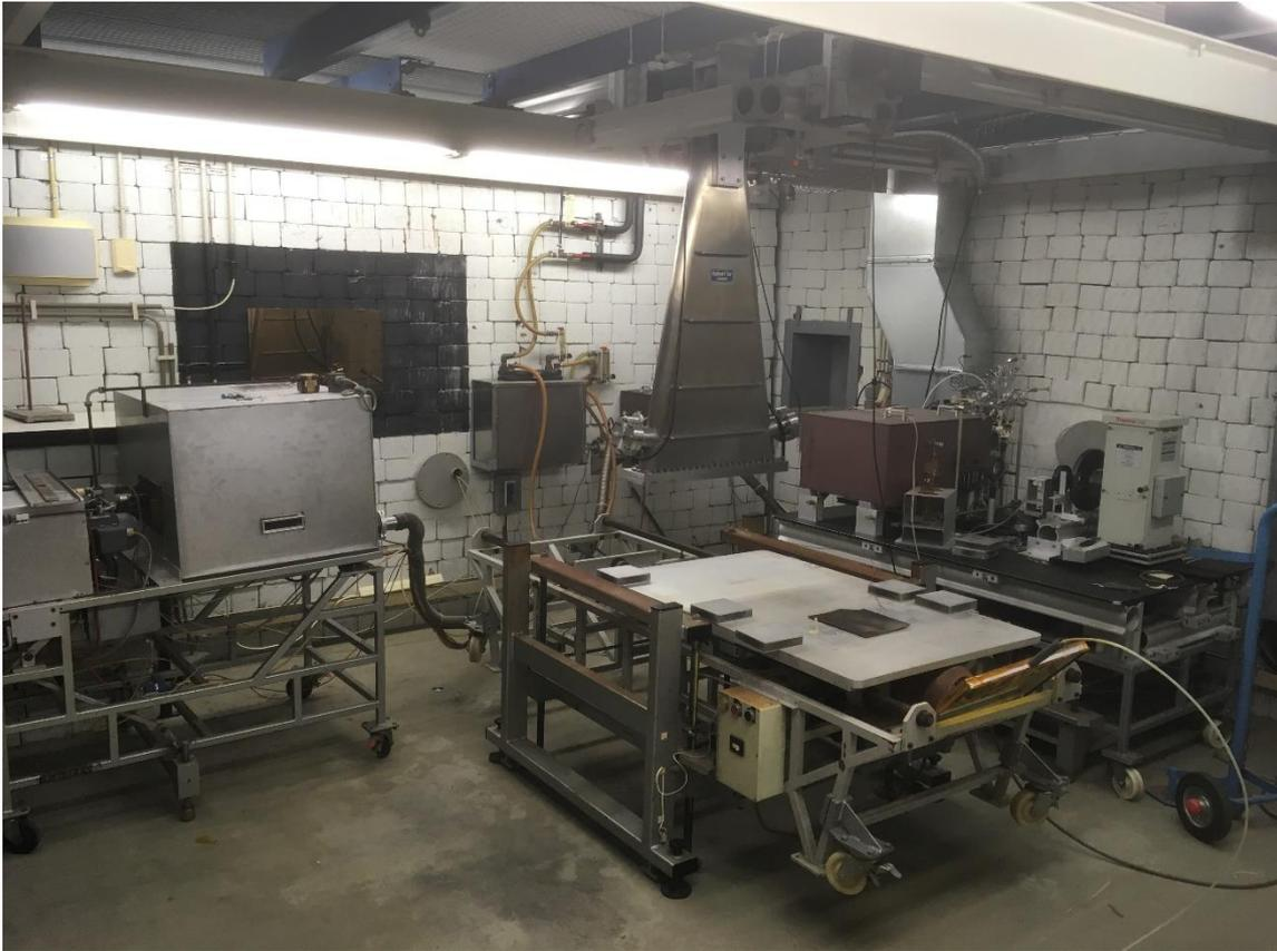
Figure 6.3: Test bed of the van de Graaff electron accelerator
