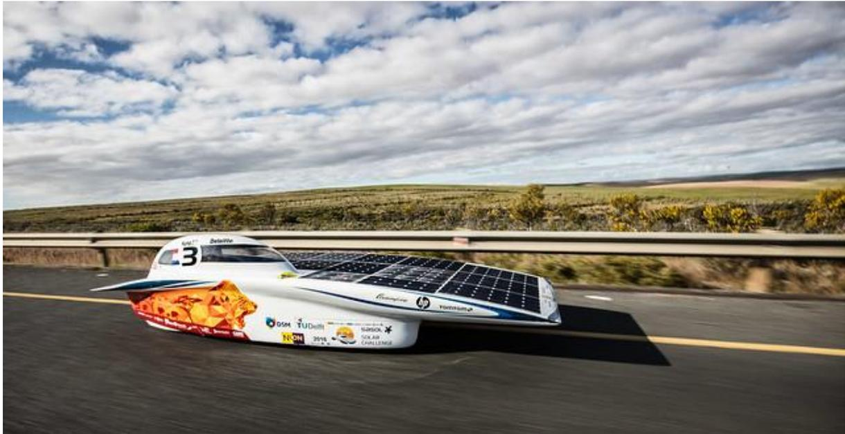
Figure 3.4: Picture of Nuna 8S, a solar powered car using Semi-flexible solar panels [4]
