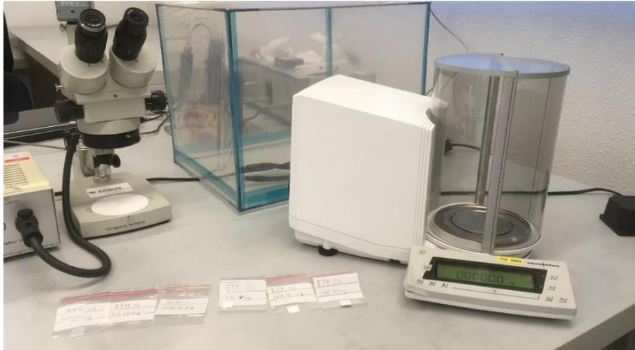
Figure 6.11: Outgassing samples and balance
