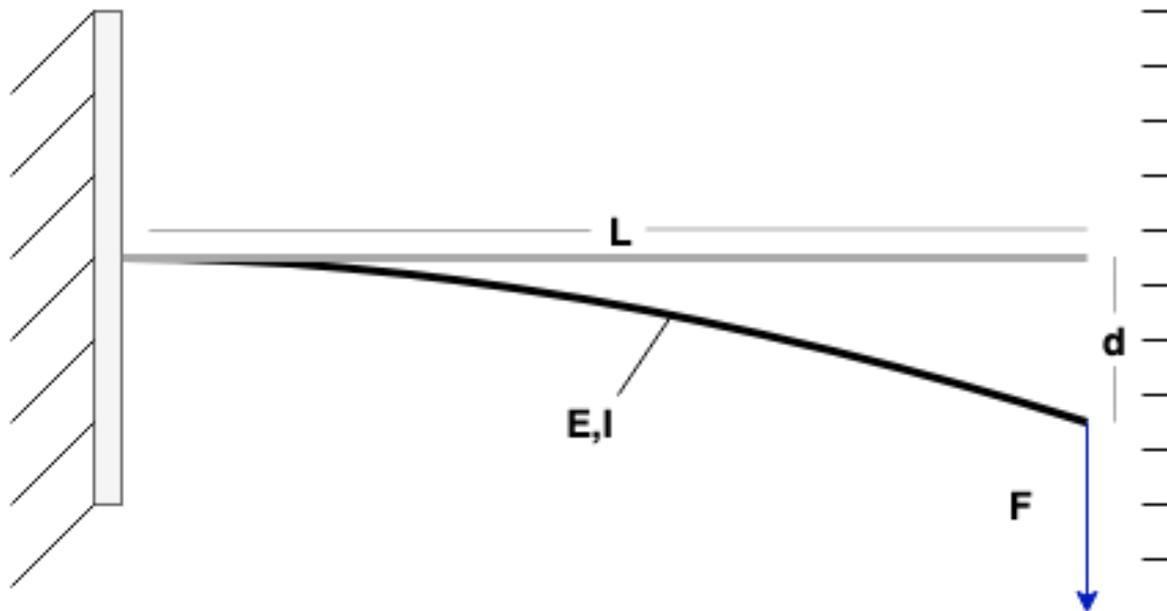
Figure 6.13: Schematic representation of stiffness measurement setup
