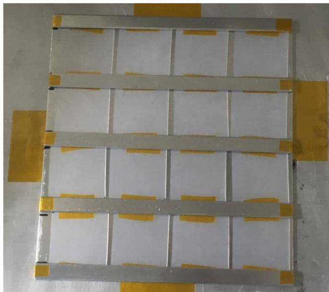
Figure 6.8: VUV degradation test samples in sample holder
