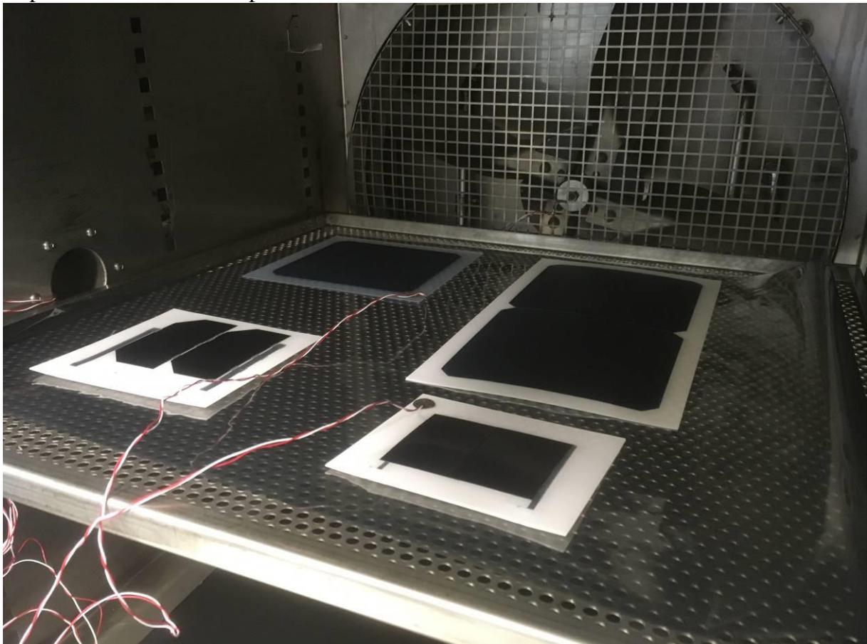
Figure 6.9: Samples in the thermal cycling chamber before cycling
