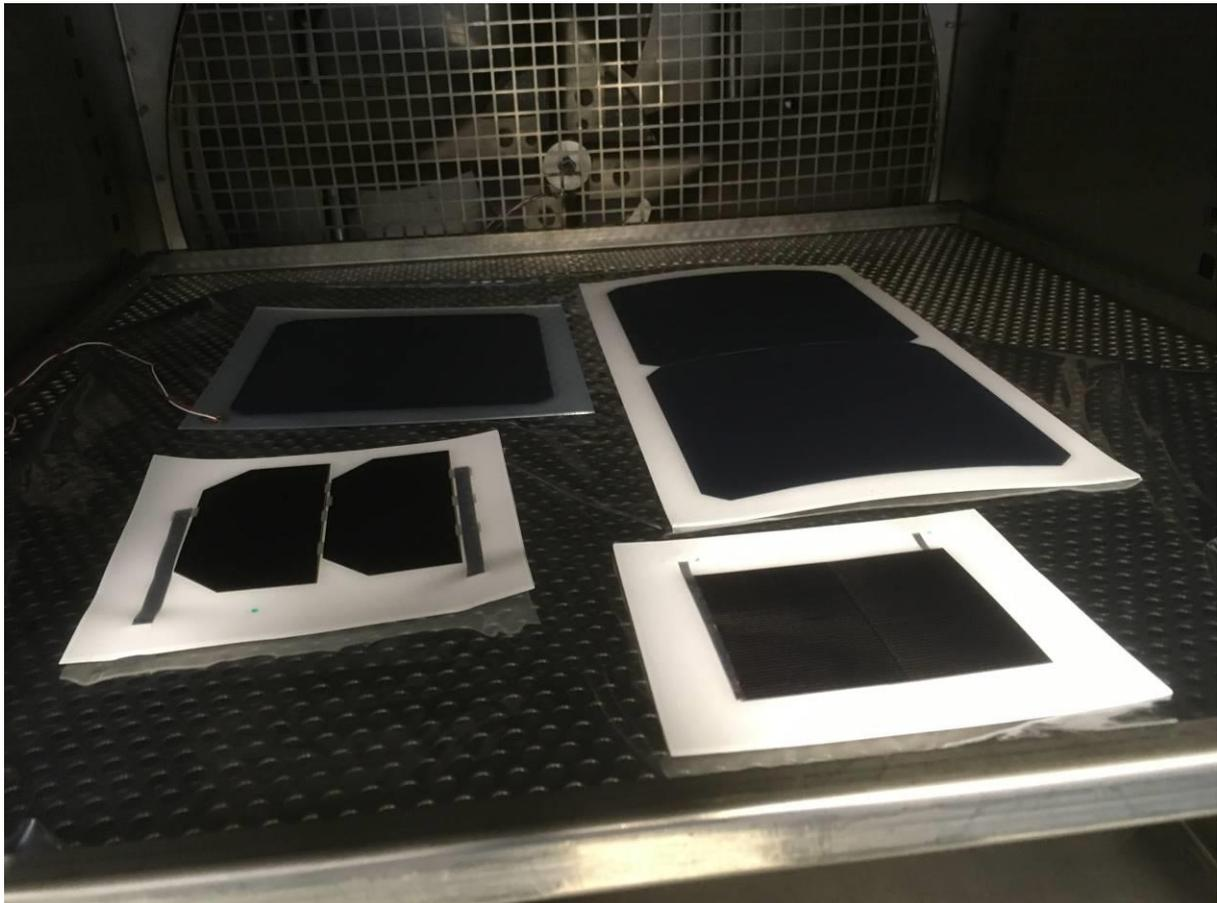
Figure 7.7: Samples in thermal cycling chamber after cycling
