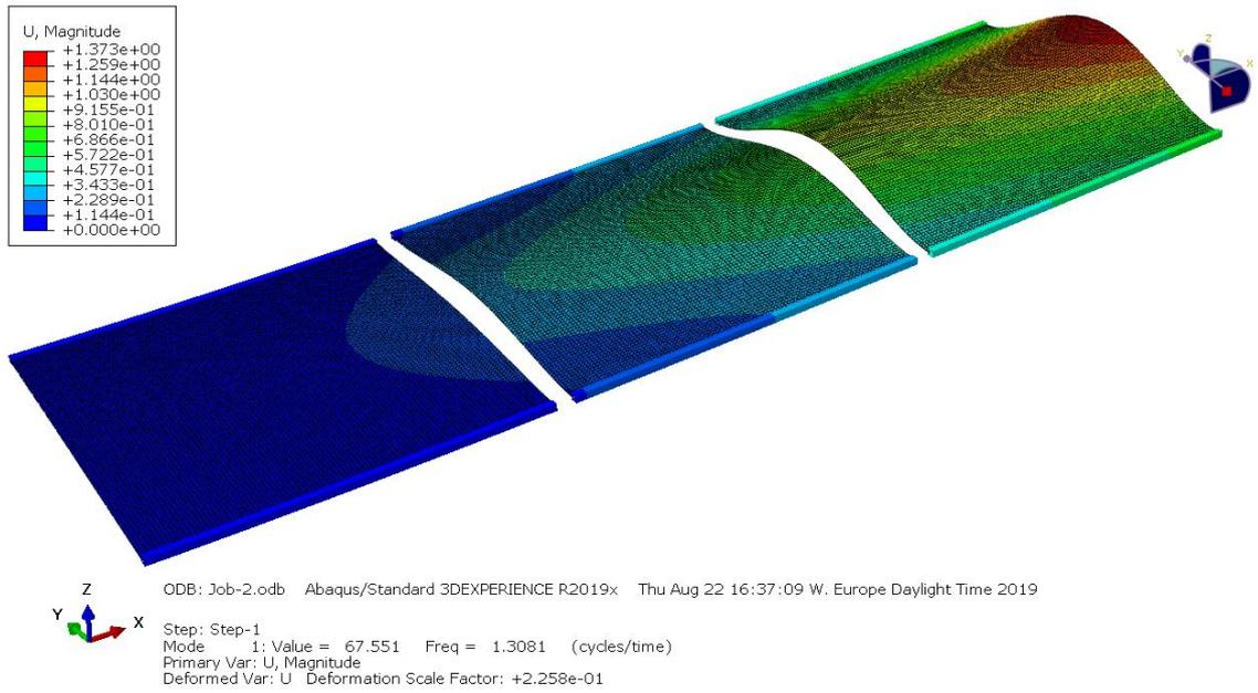
Figure 7.10: Structural analysis of case 3
