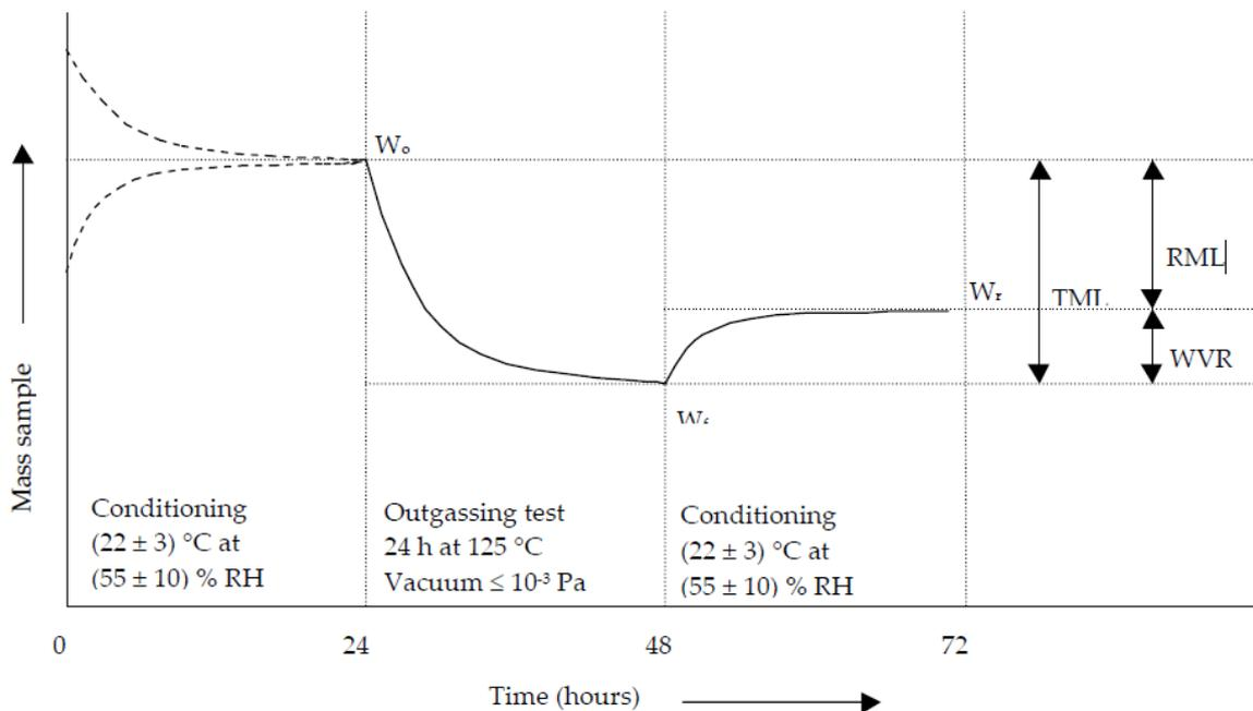
Figure 6.10: Mass change course outgassing test [14]
