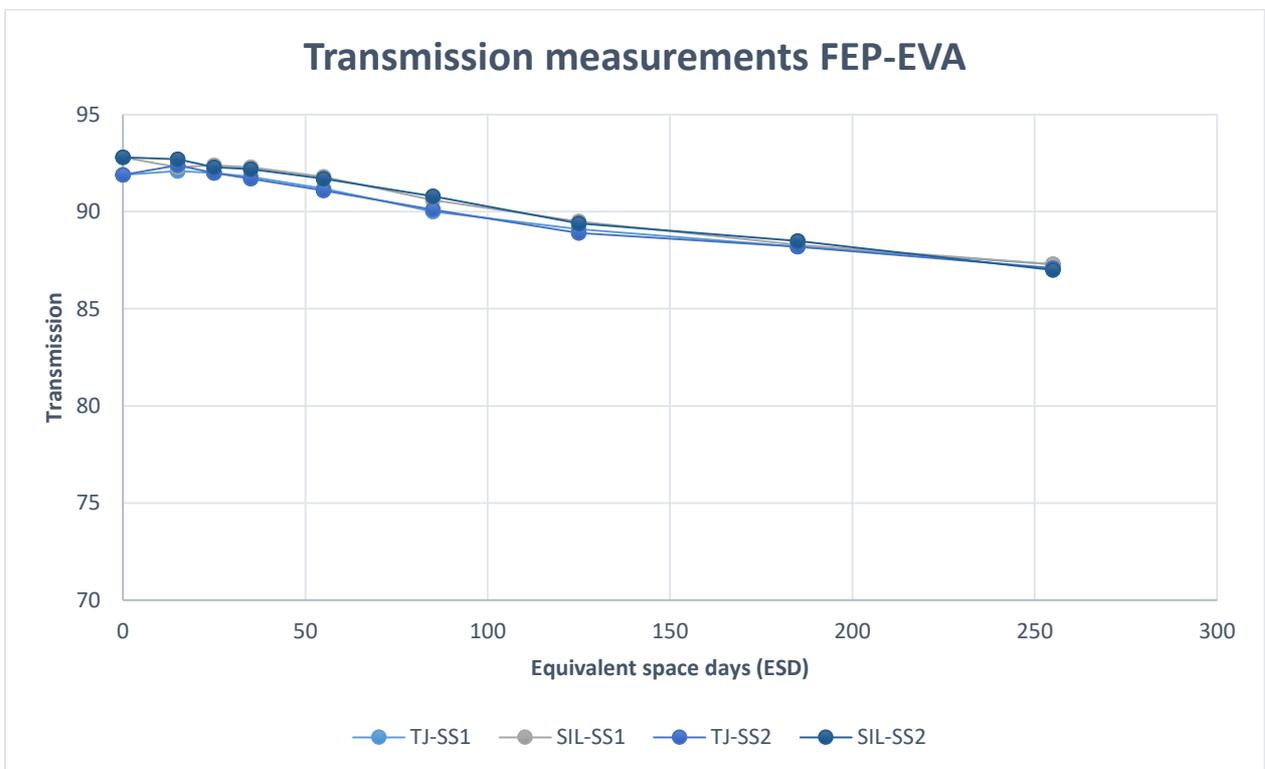
Figure 7.6: Transmission of FEP sample for a TJ and a Silicon cell as a result of VUV degradation
