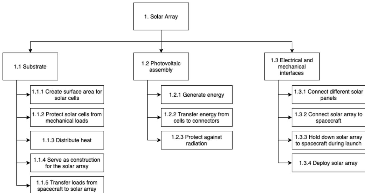
Figure 3.5: Solar array system functional breakdown diagram
