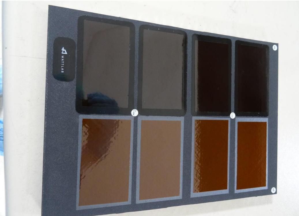
Figure A.12: Bonding of kapton on carbon face sheet rough side
