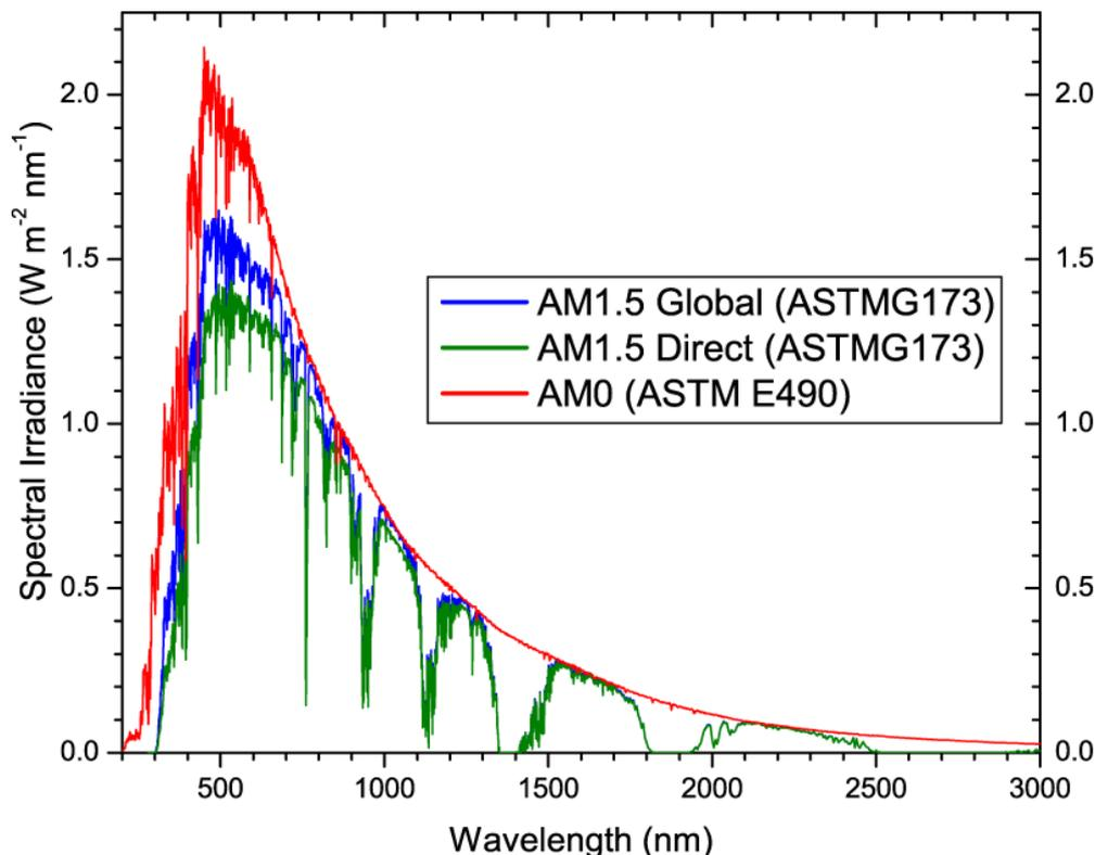
Figure 6.5: Space and terrestrial solar spectra [22]
