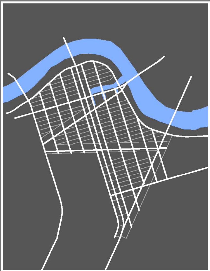
250m * 90m grid: flexible urban form north to south - mainly for Motor Vehicle north to south is the main direction for traffic of the site due to the position ( bridge area to cross the river) west to east - mainly for pedestrian
