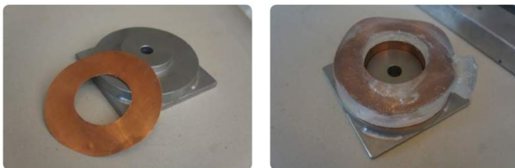
Figure 4.5 The steel endings and the copper interlayer
