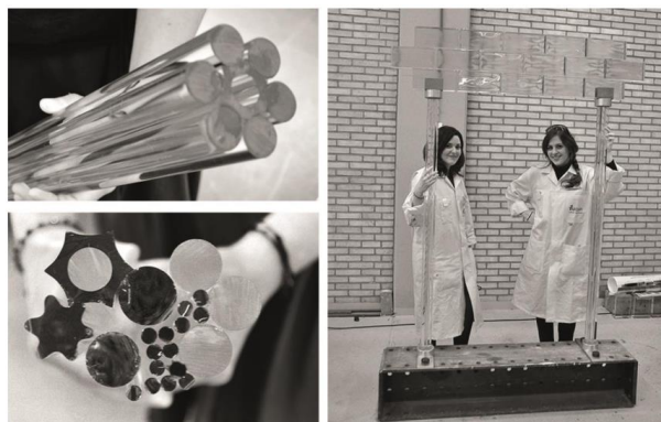
Figure 3.8 Bundles glass columns.
