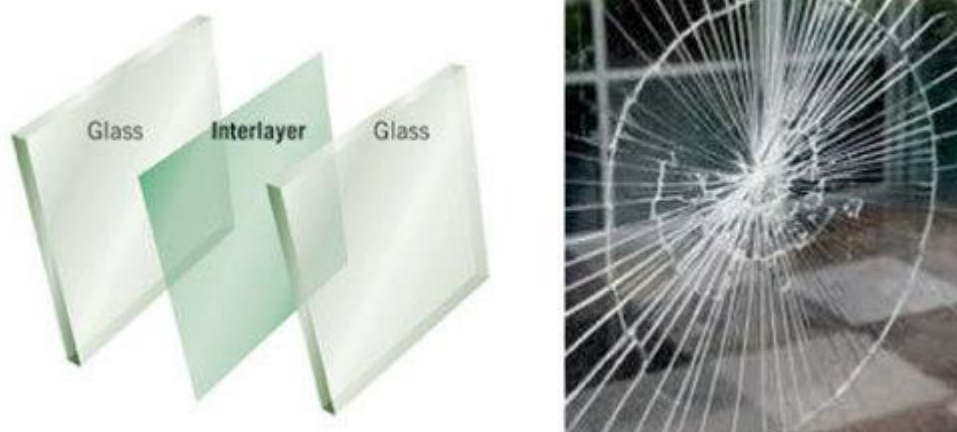
Figure 2.15 Concept of laminated glass and its breaking pattern
