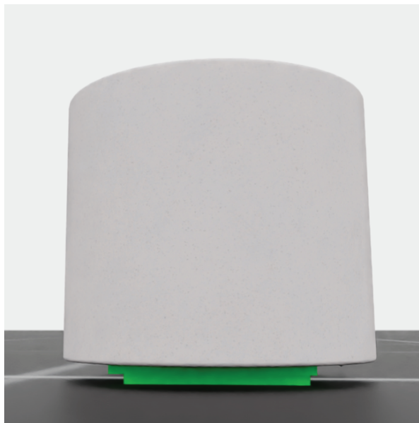
Figure A.5: Close-up view of the container and digital scale. The container sits on a simulated force-sensitive cube that records the weight of the poured liquid.
