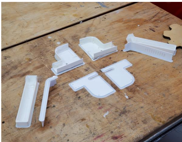
Figure 60 - FDM print of case showing the split middle case part
