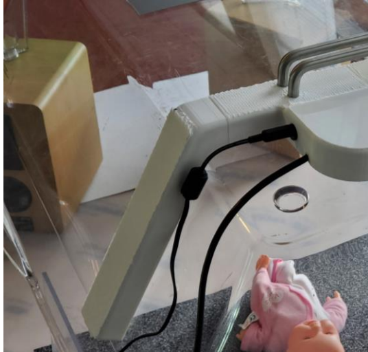
Figure 55 - Close up of prototype showing the DC barrel connector
