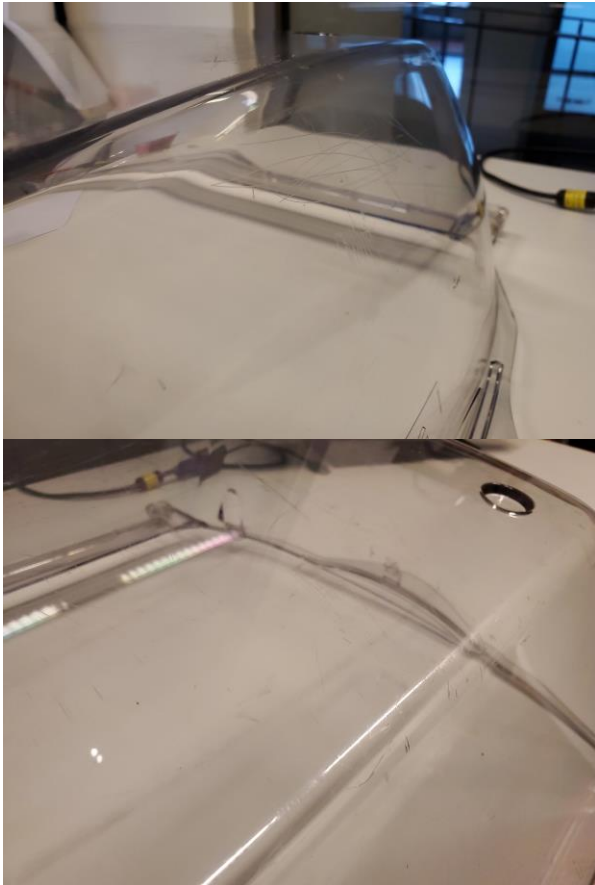
Figure 11 - Two photos showing scuffs and scratches on an incubator hood
