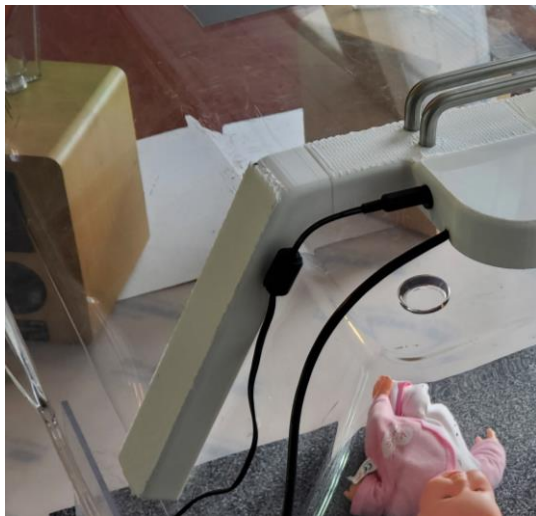
Figure 62 - Close up of prototype showing hardwired USB cable protruding from the device
