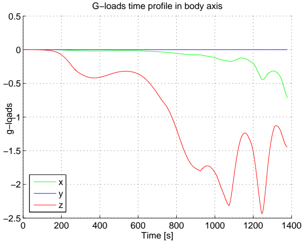
Figure 12. Lifting re-entry profiles. On the left the g -loads are displayed, showing the g -load peaks due to roll and bank maneuvers. On the right, ten Monte Carlo profiles show that the supersonic regime can be at very different pressure environments.
