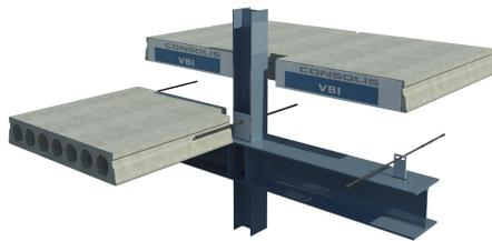
(a) Concrete and steel floor/roof system VBI hollow-core slabs [Bouwwereld, 2018].
