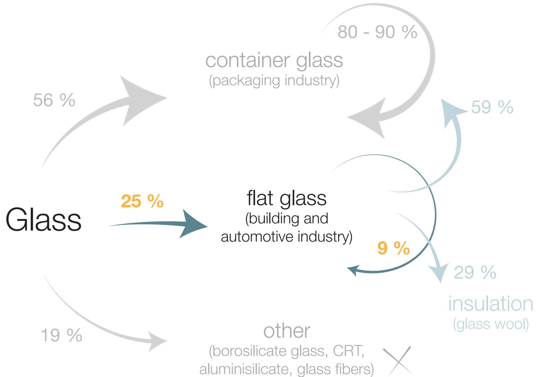
Diagram of the current glass recycling scheme in the Netherlands compared to the Re3 Glass proposal. Original From (Oikonomopoulou, 2019),
