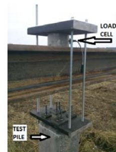
Figure 15b. Photo showing pinning of test pile to cross-beam.
