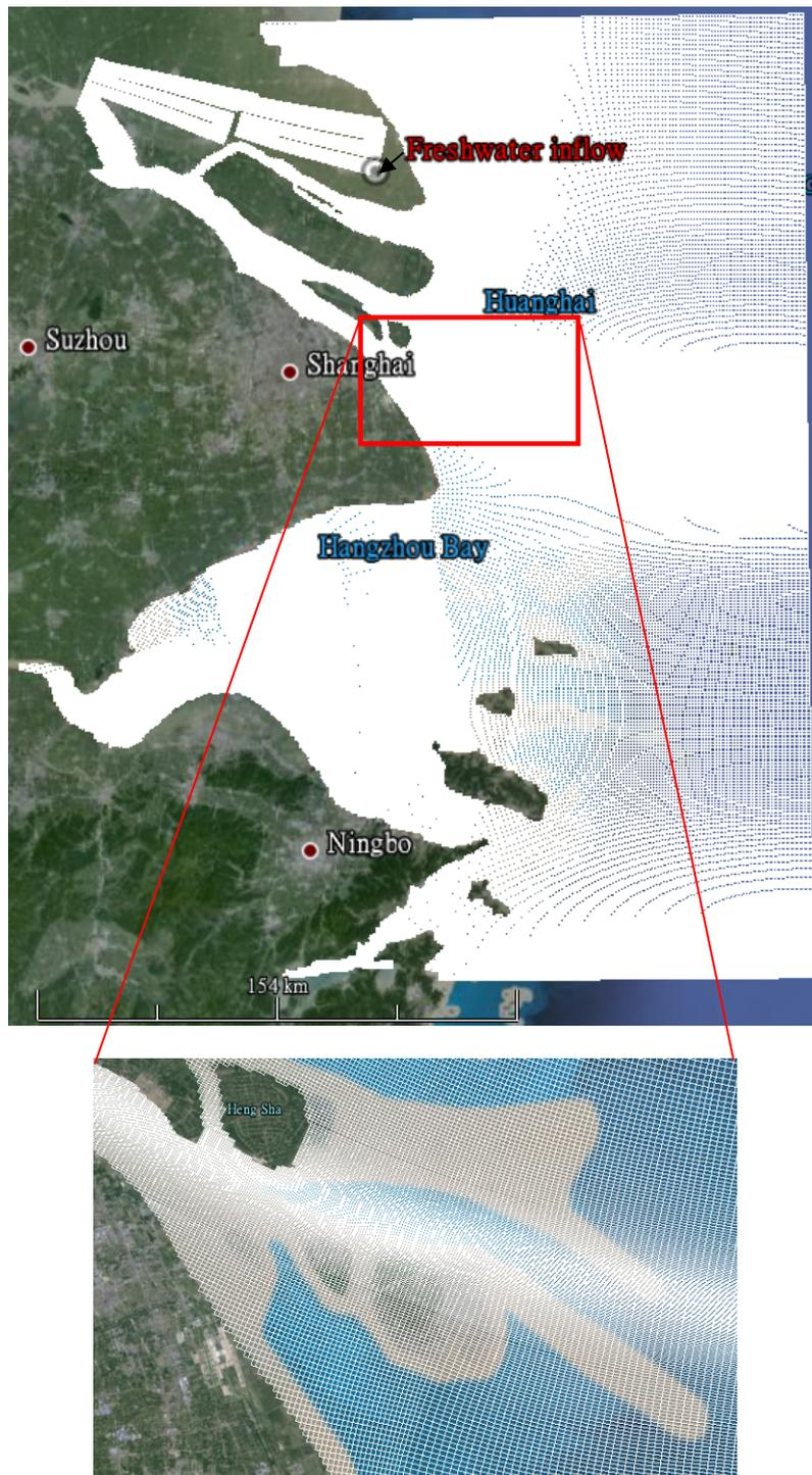
**Figure 7-13.** Google Earth based model domain and horizontal mesh (including local enlarged grid of the North Passage), upstream riverine watercourse is simplified to an N-shaped channel for preserving the conservation of tidal prism.
