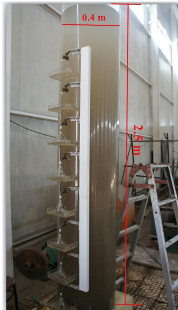
**Figure 5-1.** Photo of a traditional settling column, the outlets are connected together to a shaft to insure simultaneous sampling (Photo courtesy: *Huang Wei*).
