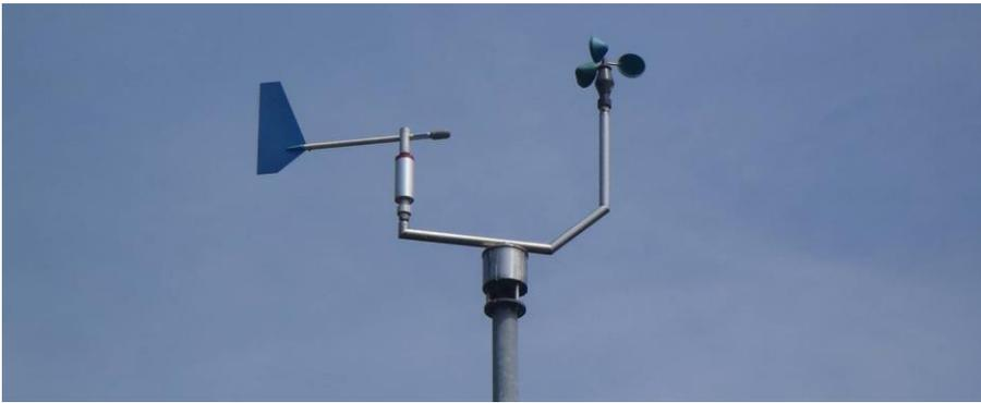
Figure 13 Left: Wind direction sensor. Right: Anemometer. Source (official website): <https://www.knmi.nl/kennis-en-datacentrum/achtergrond/recent-developments-in-knmi-s-surface-observing-methods>
