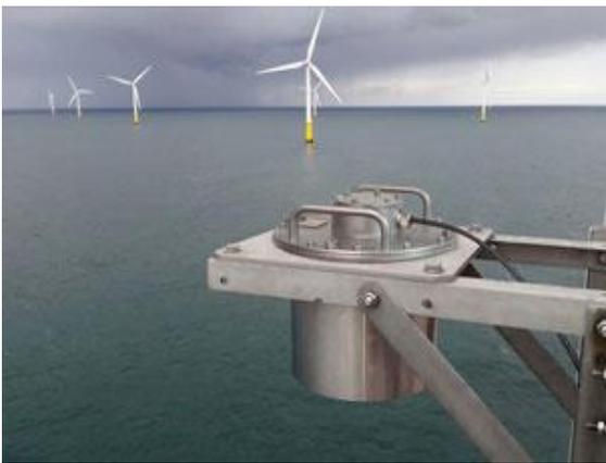
Figure 8: Left: Wave radar used to measure the raw water surface elevation time-series (Source (official website): <https://radac.nl/wave-height-tide/>).
