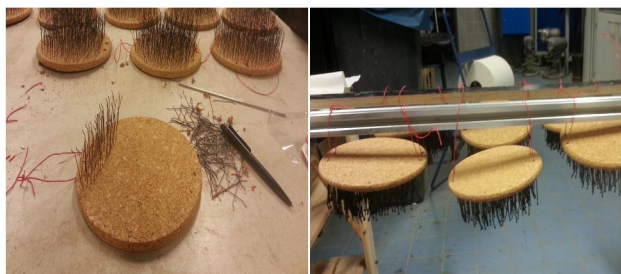
Figure 1: Bitumen coating of steel fibres.
