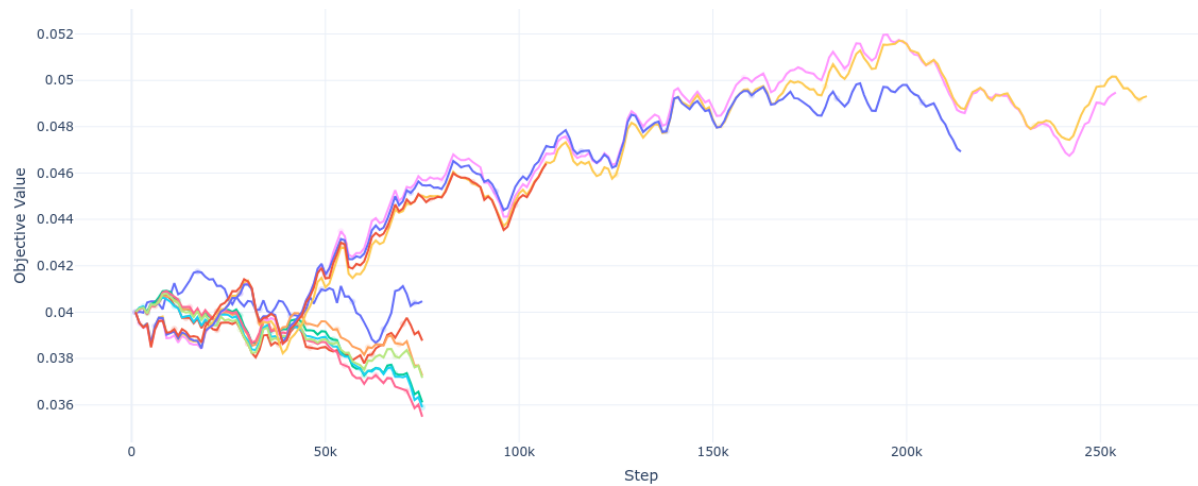
Fig. 7.5. Discrete RL fine-tuning training runs with different hyperparameters. Objective value (mean reward as performance gap w.r.t. greedy, see Section 7.1.1) over training steps (finished episodes). The previously found model (trained with discrete RL on 10 tasks, 3 robots) is fine-tuned on problem instances of 20 tasks, 5 robots, 3 skills, and 5 precedence constraints. For reference: On this problem size, the pure IL approach achieves a value of 0.08
