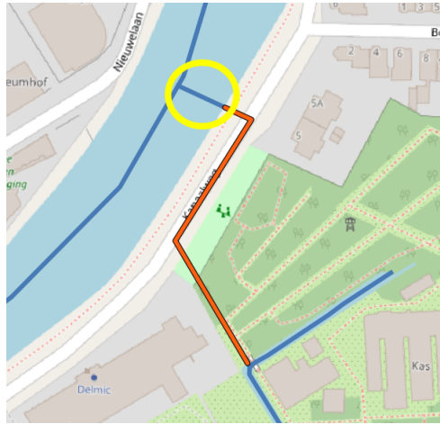
Figure 2.7: Example of pipe connecting two waterways. In orange is presented the pipe line, while in the yellow circle is shown the remaining branch
