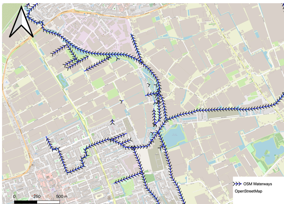
Figure 2.20: The Open Street Map waterways features displayed in blue. The direction of the geometry is displayed in black.
