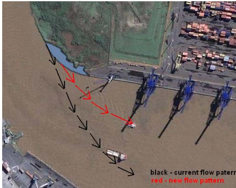
figure 12-1: flow around bend
