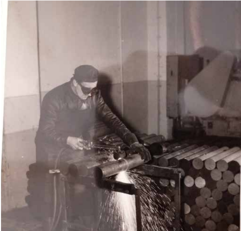
Fig. 3.5.4 Building 333 Employee cutting metal cylinders by hand with a cutting torch, that later on will be pressed into projectiles.
