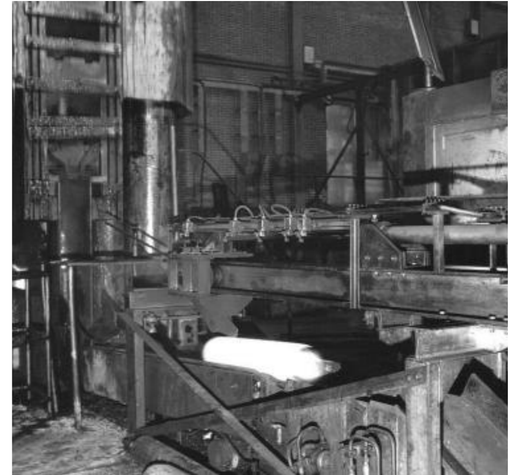
Fig. 3.5.6 Building 436 Projectile coming out of the large projectile press
