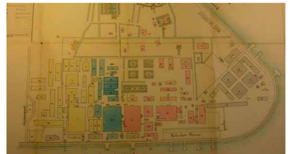
Fig. 2.2.5 3 functional zones Artillerie Inrichtingen 1924. Yellow buildings: gun factory, Blue buildings: cartridge factory, Red: ammunition factory (from SteenhuisMeurs, 2010)
