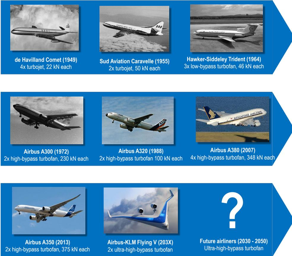
Figure 1.1: The evolving trends of jetliners. Image sources following the chronological order: [5], [6], [7], [8], [9], [10], [11], [12].
