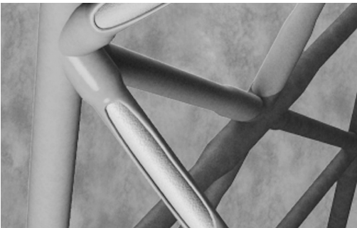
Fill the structure with concrete or grout
