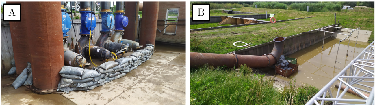
Figure 13: (A) Installed submersible pumps at the north end of the basin. The sandbags prevent clogging of the pump inlets by sedimentation of the eroded sediment. (B) Vertical pipe exit at the southeast corner of the basin to prevent large horizontal circulation in the upstream basin.
