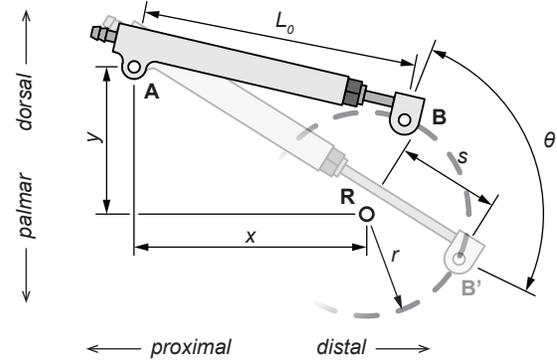
Fig. 3. Illustration showing the relation between the slave actuator's stroke ( $s$ ), initial length ( $L_0$ ) and placement of the proximal connection ( $x, y$ ) with the moment arm ( $r$ ) and resulting joint range of motion ( $\theta$ ) around the finger joint ( $R$ ).
