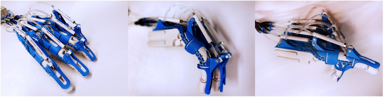
Fig. 4. Photos of the prototype fitted on a mock-up left hand with, from left to right, fully extended position, fully flexed position and pointing with index finger.
