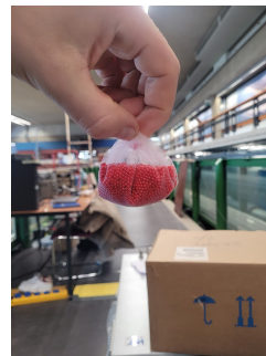
Figure 3.7: Suspended 1 to 40 1.9 mm glass spheres filled bag G1
