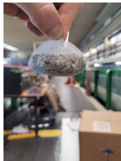
Figure 3.6: Suspended 1 to 40 narrow graded rock bag S1
