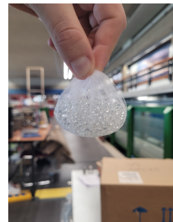
Figure 3.8: Suspended 1 to 40 4 mm glass spheres filled bag G2
