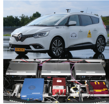
Fig. 4. TNO Renault Grand Scenic (2018) testing platform.
