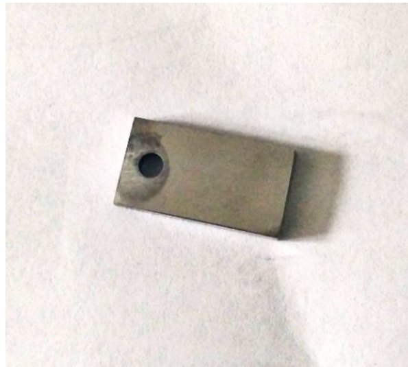
Figure 2.1: Fe-3%Mn ingot; unpolished
