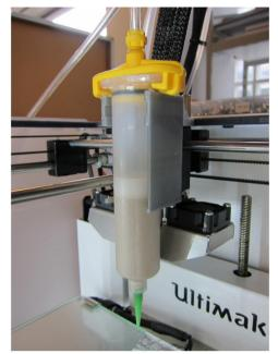
Figure 5.3. Extrusion printing setup
