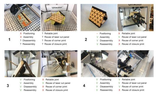
Figure 4.3. Four iterations in the prototyping process are shown. For each iteration, we evaluated the prototypes on manufacturability (ease of positioning and assembly), dis- and reassembly, robustness, and reuse of parts. We conducted several artefact iterations to explore the new circular digital fabrication workflow in practice.
