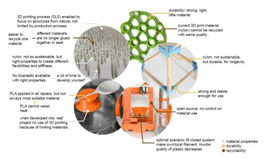
Figure 3.15. Annotations related to the material input of additive manufacturing.
