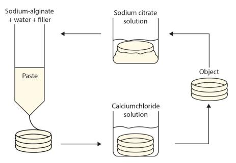
Figure 6.3. (Re)printability process based on ion cross-linking
