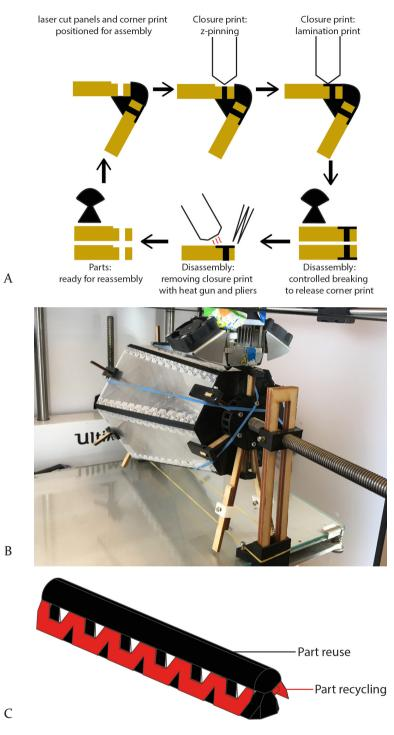
Figure 7.2. A: procedure to create reversible joint. B: parts are fixed in a clamp for assembly by 3D printing. C: Part of joint suitable for reuse (black) and recycling (red).
