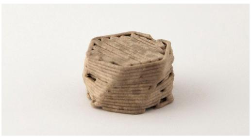
Figure 5.4. Result of material extrusion with recycled material.
