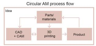
Figure 7.1. Circular AM process flow.
