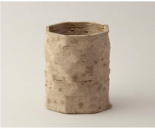
Figure 5.5. Flowerpot printed with mussel shell material.
