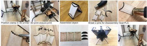
Remove PLA with pliers Clean laser cut parts All parts ready for reassembly Position parts into clamp Position clamp in 3D printer
