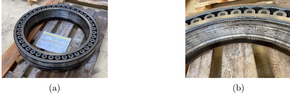
Figure 3: (a) Corroded bearing from Steyr, bearing B. (b) Closer look of Corroded bearing from Steyr.
