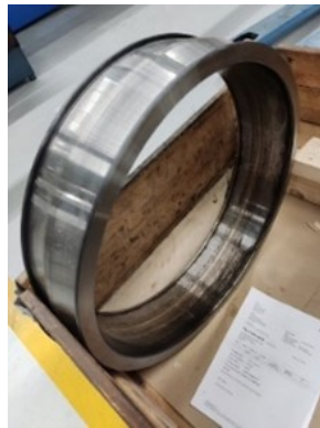
Figure 2: Slightly corroded bearing from Steyr, bearing A.
