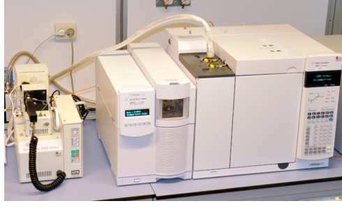
Figure 6: CDS Analytical Pyroprobe 5000 system. Equipment used for the Thermal Desorption Analysis (TDA).
