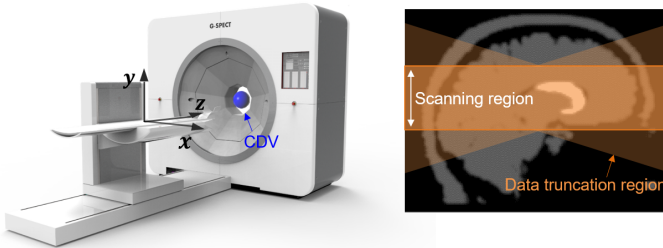
Figure 5.1: Illustration of the G-SPECT-I scanner (the left image) when a small-bore collimator dedicated for brain imaging was mounted, and the focused striatum imaging strategy (the right image). The CDV is the volume “seen” by all pinholes; it has a transaxial diameter of 100 mm and an axial length of 60 mm. The patient bed can be shifted in xyz directions to position different parts of the patient head into the CDV and thus extend the scanning region with sufficient sampling. With the focused striatum imaging strategy, the scanning region is confined in axial direction to maximize the count yield from the striatum. The data truncation region is ‘seen’ by only part of the pinholes and thus sampling is not complete.
