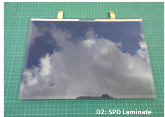
Fig. 7 Photos of the switchable glazing samples – Solar-PDLC (Left); SPD (Right). *** ** Photos not taken on the same day as that of the experiment
