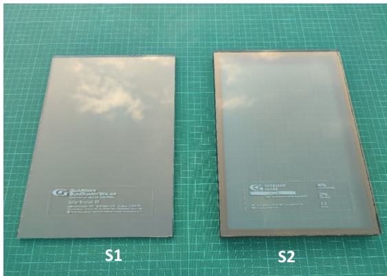
Fig. 6 Photos of the static glazing samples featuring a solar control coating. *** ** Photos not taken on the same day as that of the experiment
