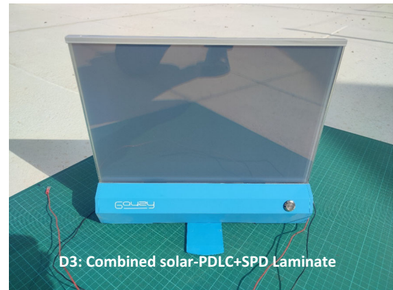
Fig. 8 View of the Gauzy-Hitachi prototype combined solar-PDLC & SPD laminate under investigation. **** Photos not taken on the same day as that of the experiment
