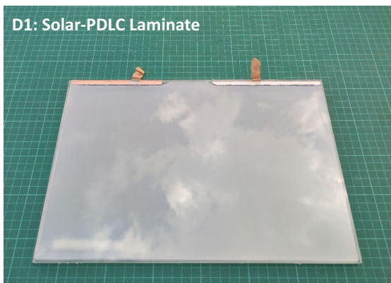
Fig. 7 Photos of the switchable glazing samples – Solar-PDLC (Left); SPD (Right). *** ** Photos not taken on the same day as that of the experiment
