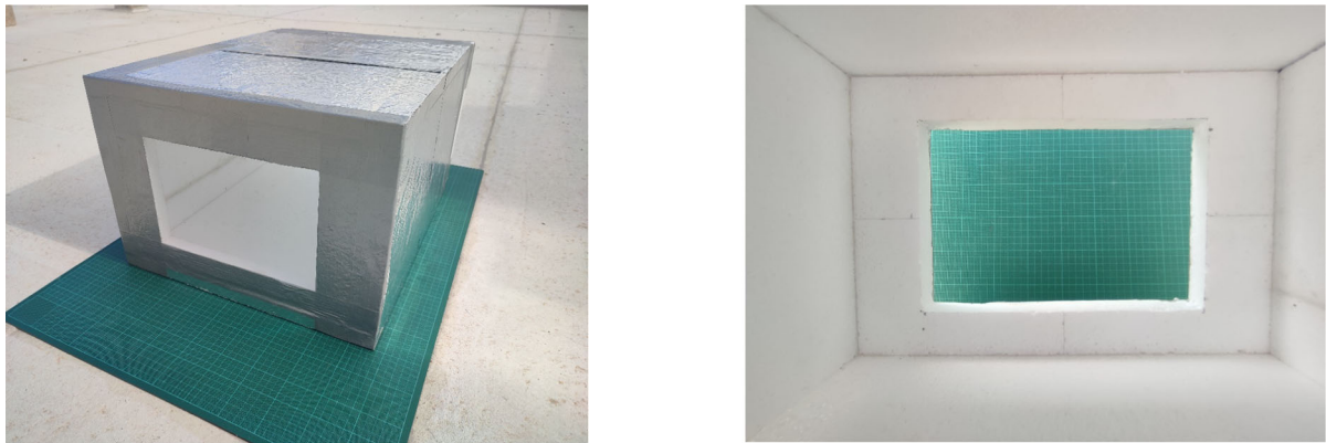
Fig. 3 External and internal views of the scale model used for the luminance field experiments
