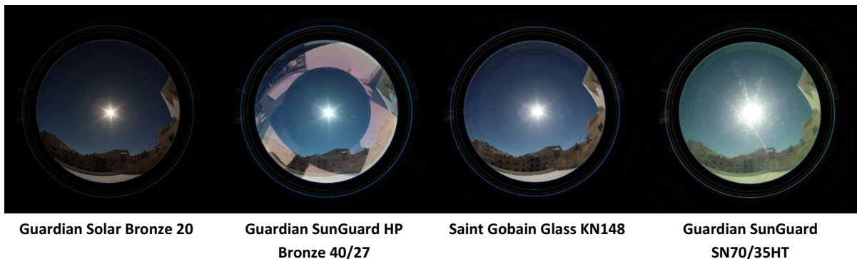
Fig. 10 Photographic fish-eye shots of the solar disc as seen through the reference glass samples
