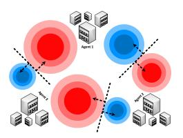
Figure 2: Idealized three-building ATES case study. Each building has a single ATES system which consists of a warm and a cold well. Warm and cold wells are shown with red and blue circles. The unwanted mutual interactions between ATES systems are shown via black dashed lines. Figure is taken from [10].
