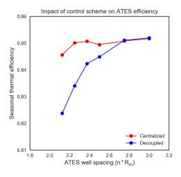
Figure 3: Simulated thermal efficiency of ATES systems with centralized and decoupled control, as a function of the distance between ATES wells (defined as a multiplier of the thermal radius Rth). In the reference decoupled case, thermal interferences degrade efficiency at smaller distances.
